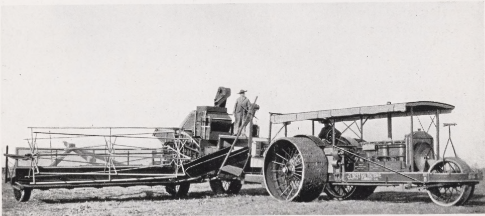
Front Side View of "C. L. B." Electric Combined Harvester
