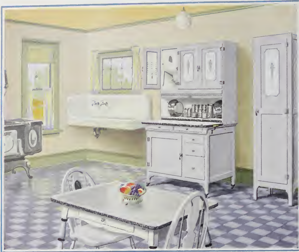
In the kitchen much depends upon the correct placing of the necessary items of equipment, such as table, refrigerator, cabinet, sink, and storage closets. The right relation of these speeds up routine work and makes for an unbelievable saving of steps. With the stove, cabinet, and sink forming a triangle, storage closets can be easily grouped near, reducing labor to a minimum.
