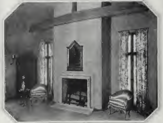
Above and left. The owner's bedroom. The heavy oak beams here and throughout the house were cut especially for this work in the same county—Allegheny—where the house stands. They were then treated with acid to give them the appearance of natural gray weathered oak, which is extremely effective against the rough plaster walls
