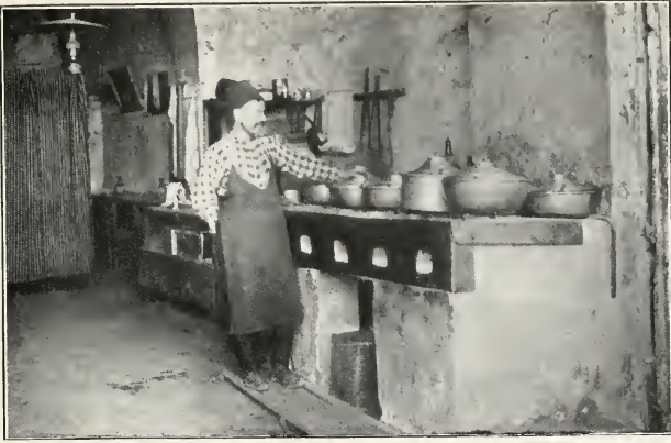
In the Turkish restaurants food is cooked over holes in a limestone slab, while below the charcoal fire is fed through other openings which also make the draught.
