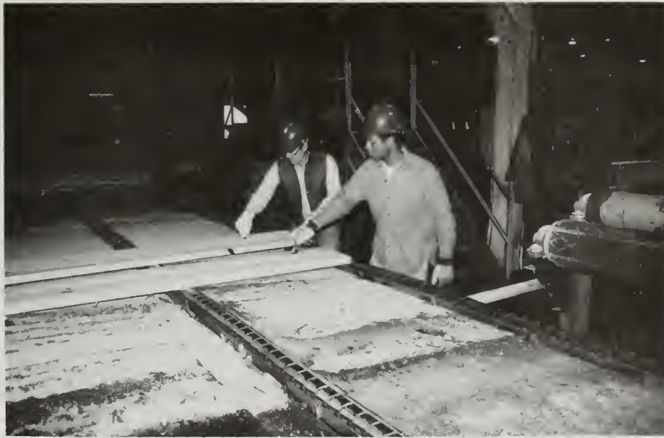
Maintaining the identity of lumber produced in the sawing phase of mill recovery studies is also a critical part of the study.
