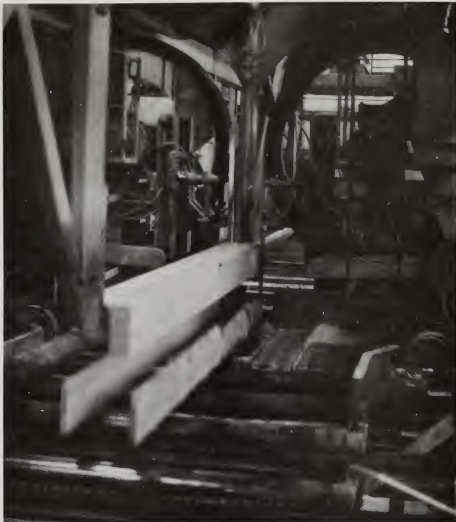
This double-bandsaw headrig with an end-dogging carriage is one example of innovative technology used in western sawmills.
