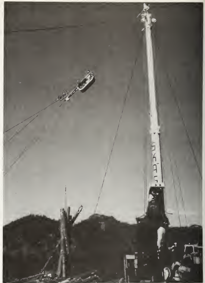
A Skagit tower with a high lead carriage system being used in steep terrain.
