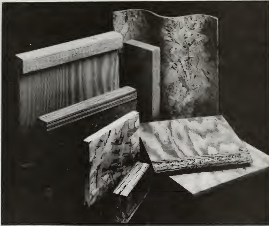
Examples of structural composite products, from top left: wood joist with laminated veneer lumber (LVL) flange and plywood web, wood joist with LVL flange and wood particle web, waferboard and subfloor/underlayment, Parallam (reg. trademark of McMillan Bodel Inc.), conventional plywood, COM-PLY (reg. trademark of the American Plywood Association), LVL, and Waveboard (reg. trademark of the Alberta Research Council). (Credit: Forest Products Research Society)
