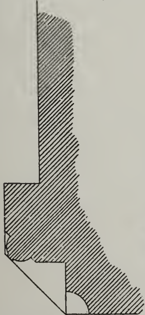
Plan of jamb 1 1/2" scale
