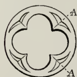
A A. The eyes of a quatrefoil.
