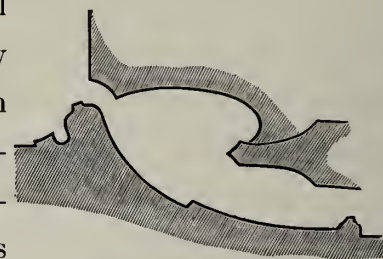
SECTION OF JAMB AND SILL.
