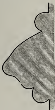
BAND TO NAVE-PIERS. PERPENDICULAR.
