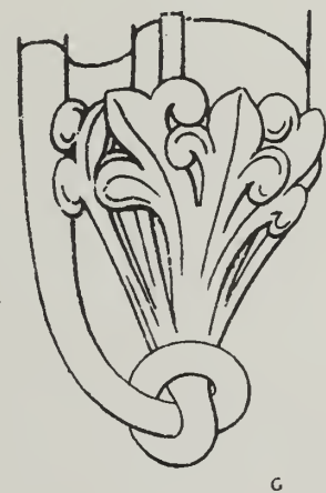
Dripstone terminations from. A. Swaton Church. Lincolnshire. B. St. Margarets Chapel Herefordshire. C.D.E. Debenham Church Suffolk. F. Monastic building, L. Winham, Suffolk. G. St. Cross Winchester. H. Westminster Abbey Church.
