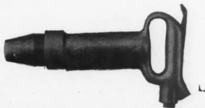
Fig. 3.—Counterbalanced Pneumatic Hammer for Calking, Chipping and Light Riveting.
