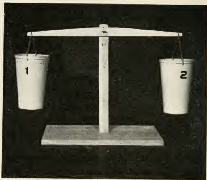
FIG. 23.—Home-made Balance Used to Show the Effect of a Dry Earth Mulch.
