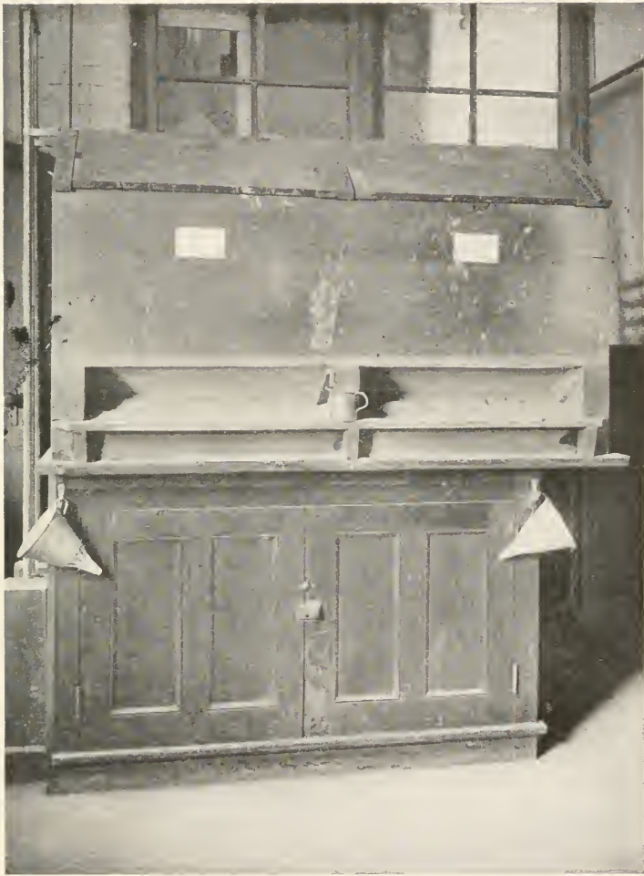
FIG. 4.—A Convenient Soil Bin, Mounted upon a Cupboard. The bins are filled from the top, the soil being removed from the open throat at the bottom. A sloping board just above the opening directs the soil back and prevents it from escaping faster than it is used.
