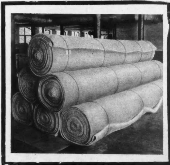
Kenwood Woolen Dryer Felts, each weighing over 1000 pounds.
