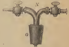
FIG 78 The Stopper and Cocks supplied with apparatus No. 2.
