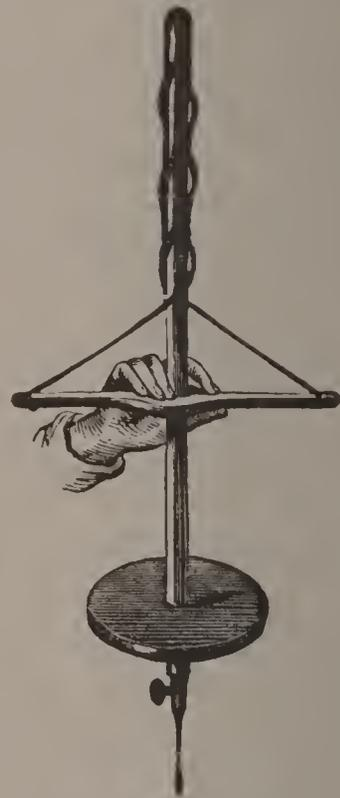
Fig. 3.—Pump Drill.
