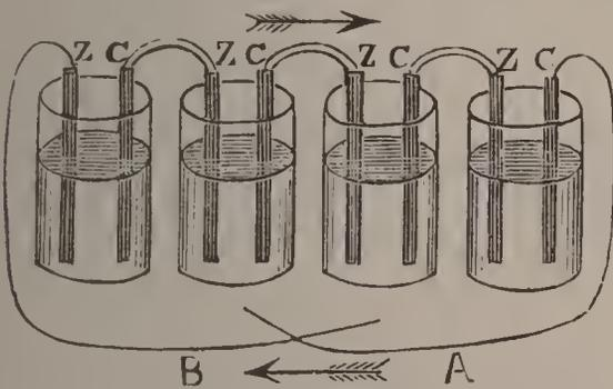
Fig. 7.—Voltaic Battery.
