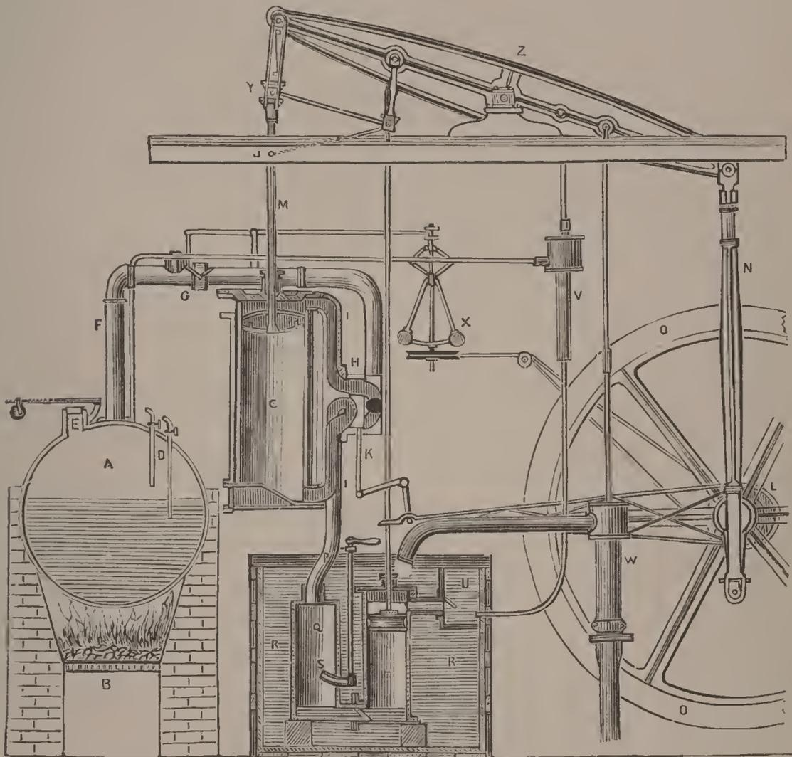
Condensing or Low-Pressure Steam Engine.
