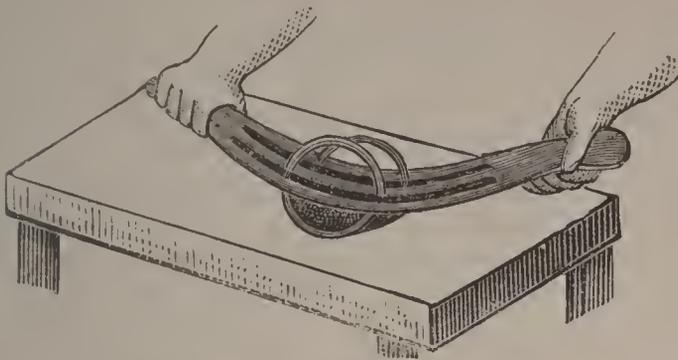
Fig. 1.—Straightening the Wires.
