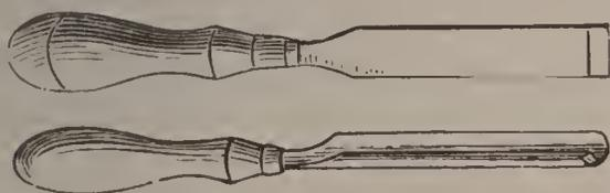
Carpenter's Chisel and Gouge.
