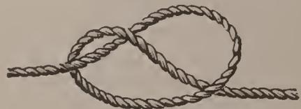
Fig. 1.—Overhand Knot.
