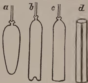
Fig. 5.—Making Cylinder Glass.
