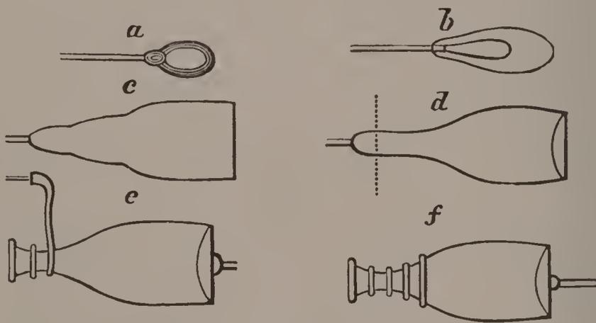
Fig. 3.—Making a Decanter.
