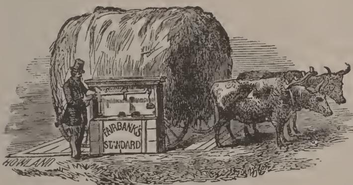
Fig. 7.—Platform Scale.
