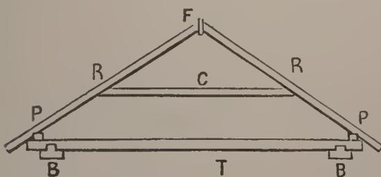
Fig. 4.—Collar Roof Frame.
