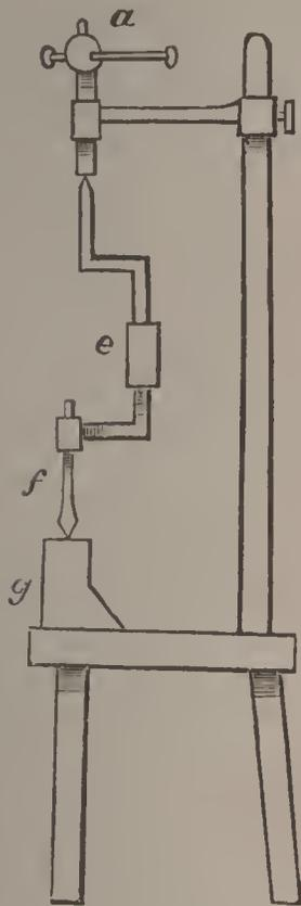
round by the hand of the workman, and the drill, *f*, is kept pressed tightly on to the piece of metal, *g*, into which the hole is to be drilled, by turning the screw, *a*, at the top. Besides these, there are machines for drilling, some of which are worked by hand and some by steam-power. As there is much rubbing or friction in drilling
