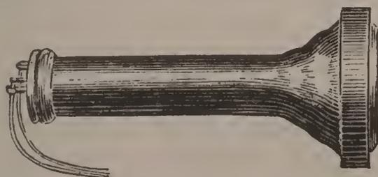
Fig. 3.—Mouthpiece of Telephone.
