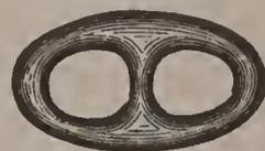
hammered together when white hot, at the ends, the stay-piece, which is of cast iron, being first put in place. The largest chain cable ever made was for the Great Eastern. The links are about as thick as a man's wrist ( $2\frac{7}{8}$  inches).
