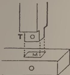
and T the tenon. When the tenon is put into the mortise, a wooden peg is usually driven through both, which keeps the tenon in place so that it cannot be pulled out. This kind of joint is much used by house carpenters in putting together the frames of houses, and in making doors, shutters, and blinds. Most of the locks on doors are fitted into mortises.
