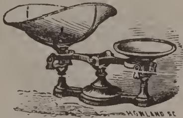
Fig. 3.—Grocers' Even Balance Scale.
