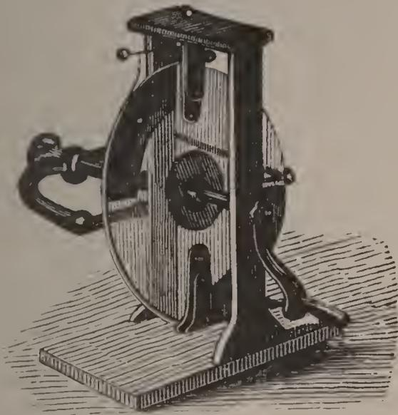
Fig. 3.—Plate Electrical Machine.
