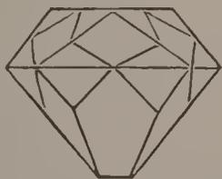
Fig. 3.—Brilliant-cut Diamond—Side View.
