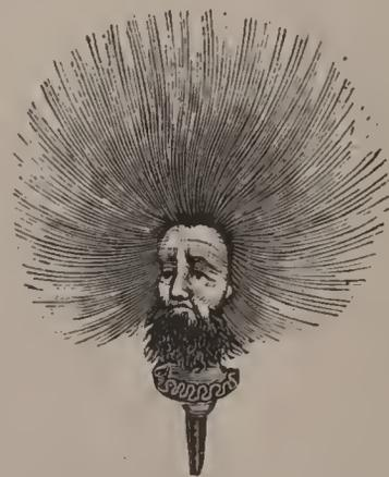
Fig. 4.—Electrified Head.
