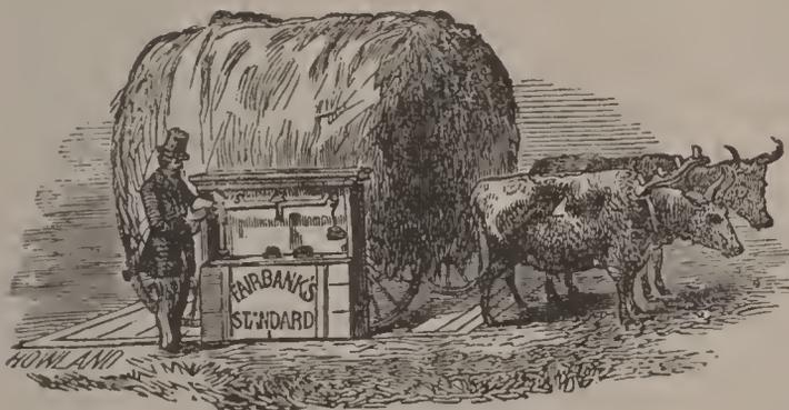
Fig. 7.—Platform Scale.
