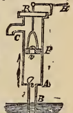
Suction Pump, viewed in section. AC Cylinder or Barrel; AB operate by a handle or lever, as if by a pump handle; as, to pump an organ. B Bucket or Piston; E rod or Spear; D \odot Valves.
