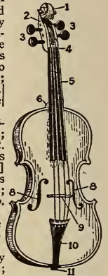
Violin (Stradivarius). 1 Scroll; 2 Peg Box; 3, 3 Pegs; 4 Nut; 5 Finger board; 6 Neck Plate; 8 Sound Holes; 9 Bridge; 10 Tailpiece; 11 Button.
