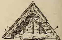
1 Bargeboard. On the right it is cut away to show 3 Bargecouple; 2 Bargecourse.
