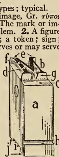
Metal Type. a Body; b Face; c Shoulder; d Counter; e Serif; f Stem; g Beard; h Nick; i Groove; j Feet.
