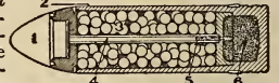
Shrapnel . 1 Combination Fuse, 2 time and percussion; 3 Steel Case; 3 Shrapnel Balls; 4 Central Tube; 5 Guncotton; 6 Strip. In general, a fragile Loose Powder.
