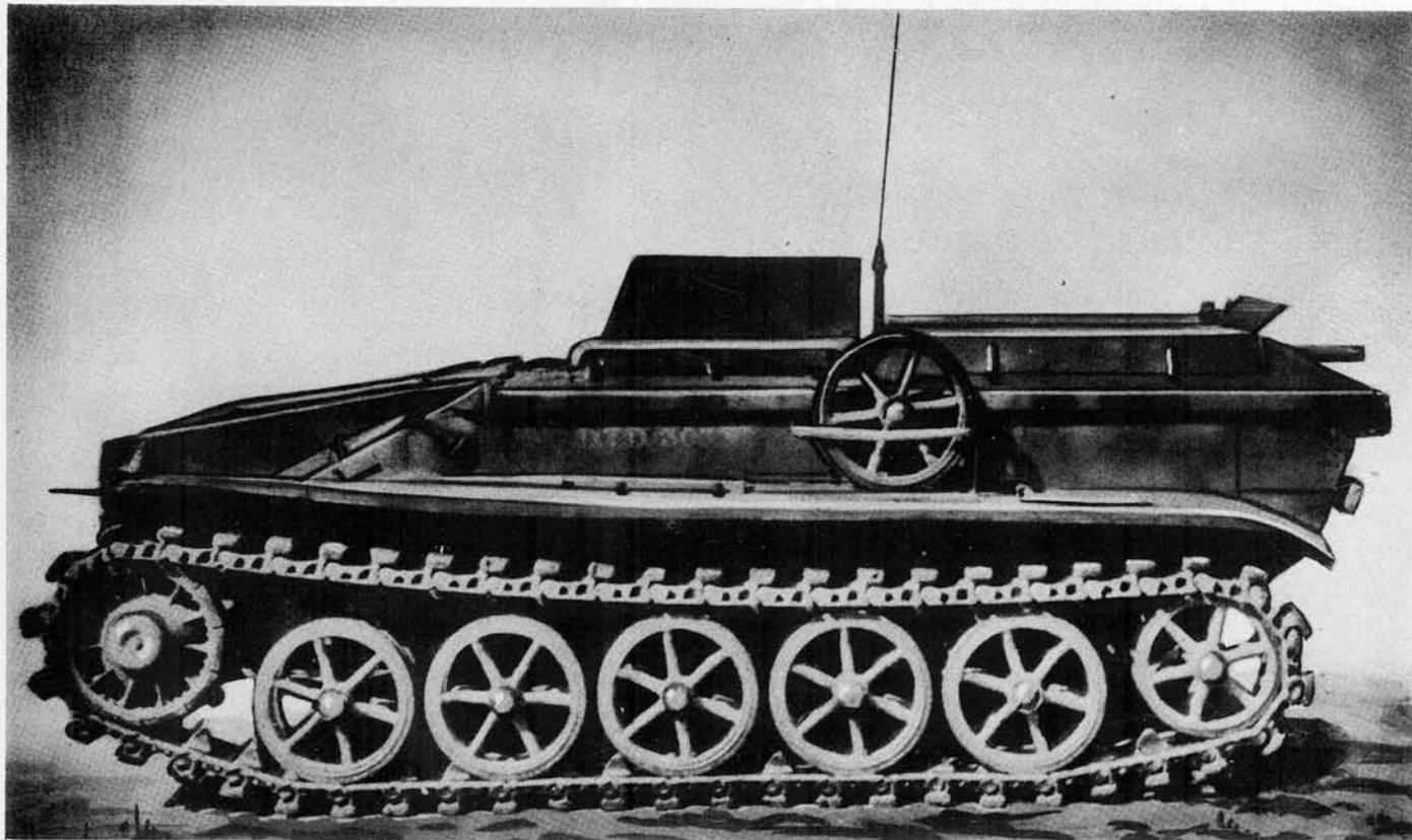
This vehicle is designed to convey a heavy demolition charge to a selected tactical objective, at which point the load may be dropped, the vehicle retracted, and the charge detonated. While it may be driven near the target, its special feature is the remote radio-control with which it may be operated after the driver leaves. Its chief use is to demolish pillboxes and strongpoints.
