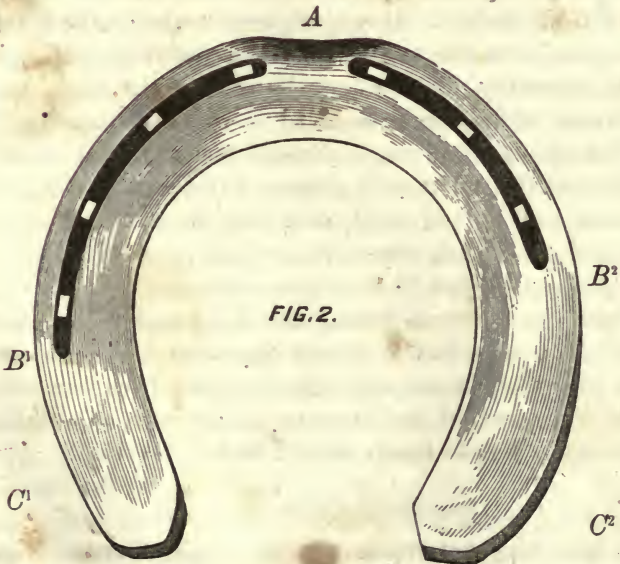
CONCAVE SEATED ENGLISH SHOE FOR OFF FORE-FOOT, SHOWING BOTH SURFACES.
