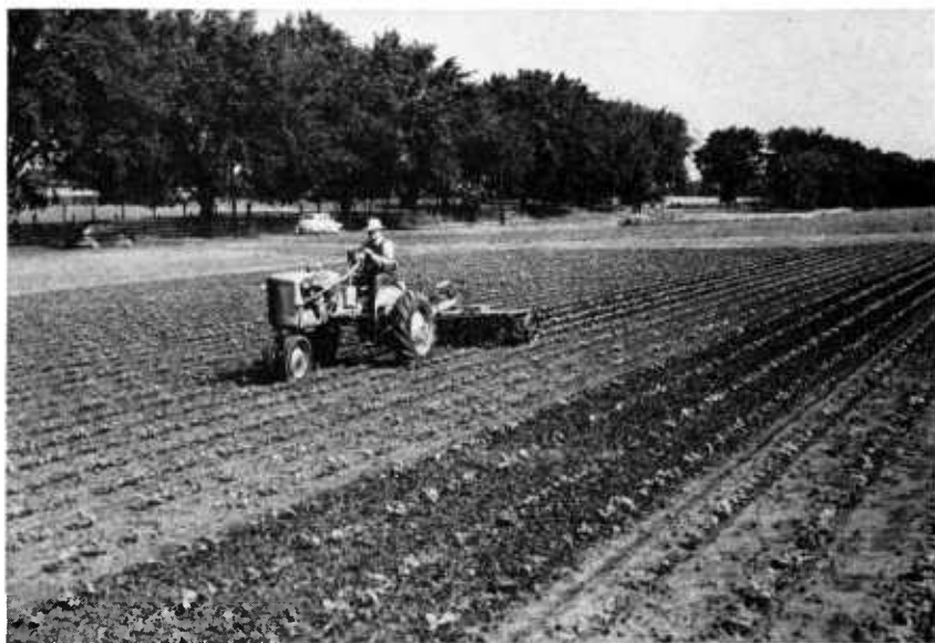
Figure 8. —A rotary hoe kills small weeds and breaks the soil crust.
