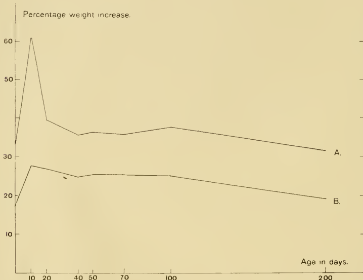
Chart 2 Showing the final percentage weight increase in two series of rats' brains, each kept for ten weeks in a neutralized solution of 4 per cent formaldehyde. A , solution made when the experiments began; B , solution five months old when used.
