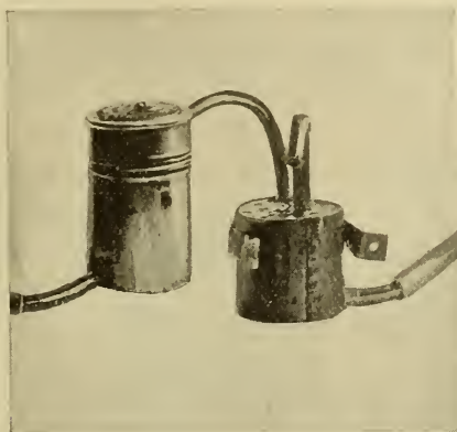
Fig. 167—The oil and water tank for the engine and boiler
