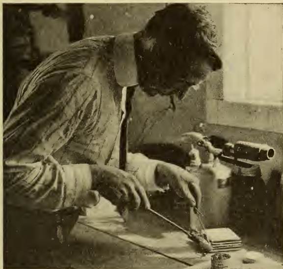
Fig. 51—Proper method of holding a soldering copper and solder
