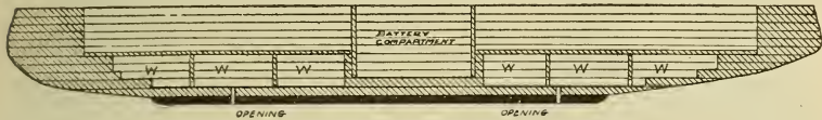
Fig. 197—Cross-section of the complete hull, showing the location of the water ballast compartments
