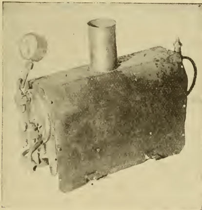
Fig. 181—The Scott semi-flash boiler used on the "Experiment"
