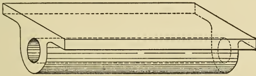
Fig. 86—Appearance of casting showing cored hole
