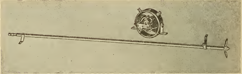
Fig. 192—The propeller shaft in the stern tube and the driving motor
