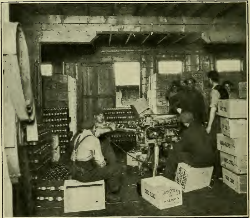
FIG. 2.—SALMON CAN-LABELING MACHINE.
