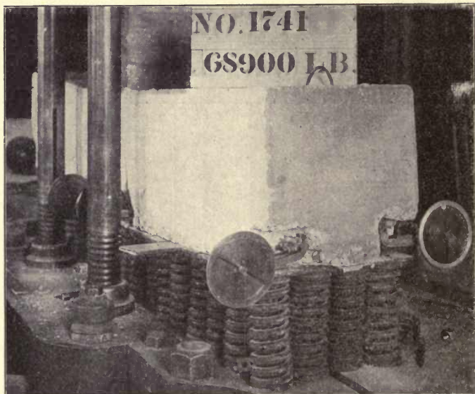
FIG. 22. INSTRUMENTS IN PLACE TO MEASURE SLIP OF BARS.
