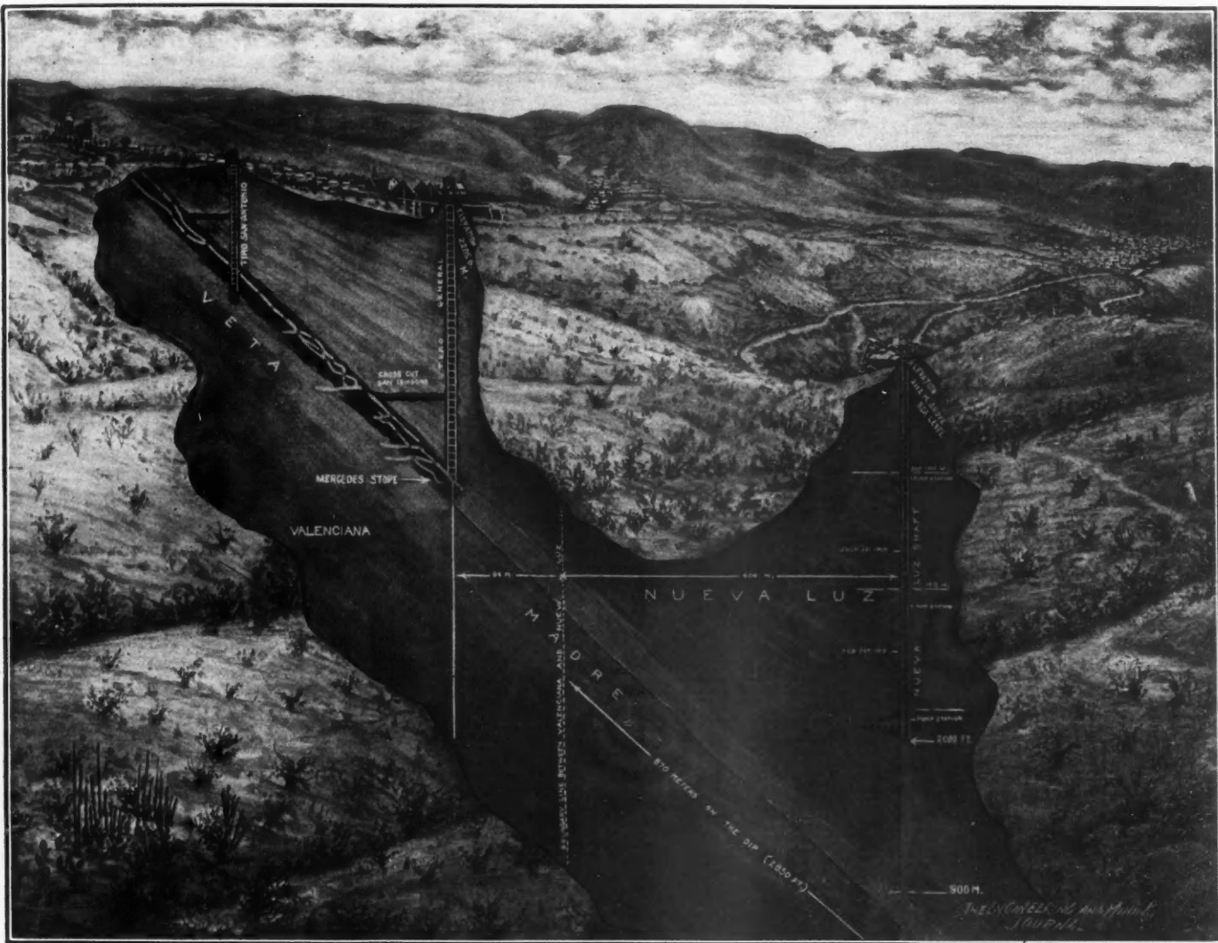
SAN ANTONIO, GENERAL AND NUEVA LUZ SHAFTS AND HYPOTHETICAL EXTENSION OF THE VETA MADRE, GUANAJUATO
