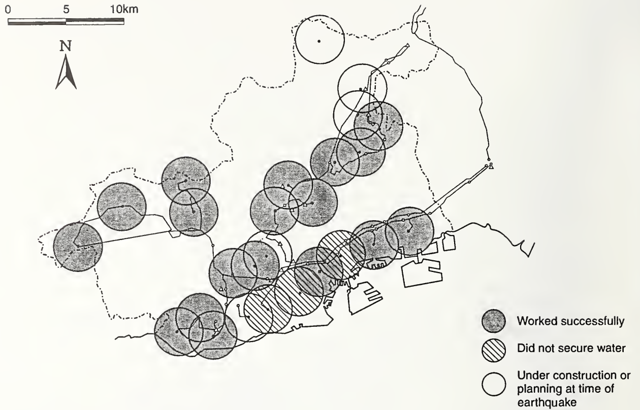
Figure 5.2.10 Map of Kobe water service area showing reservoirs with earthquake valves and their respective service area.
