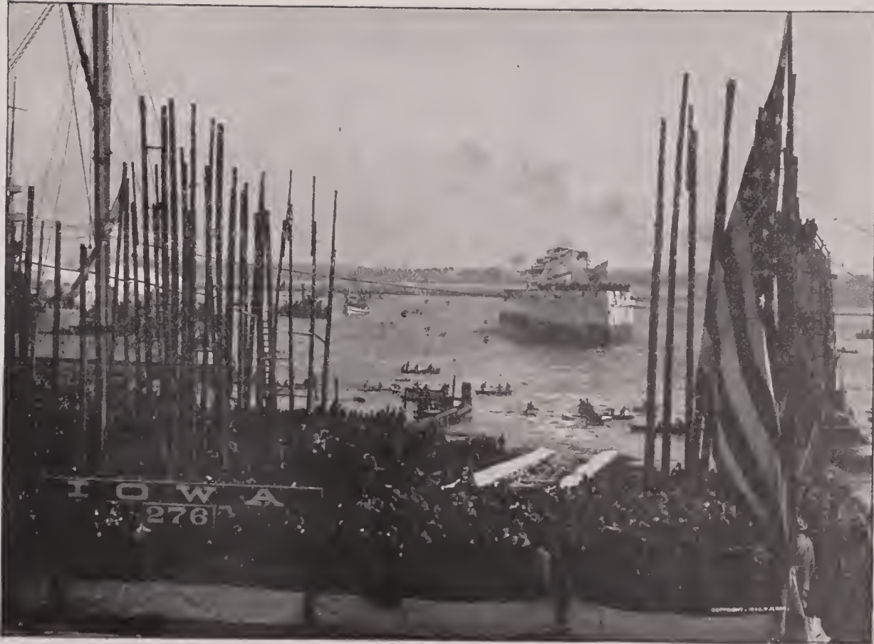
BATTLESHIP IOWA —The view here presented was taken from the shore, immediately after the Iowa left the stocks. Practically, the only part of a vessel that is complete when the launching takes place is the hull. Furniture, fittings and armaments all have to be added when the hull is afloat, but the foundation is there and a complete battleship is soon made of it
