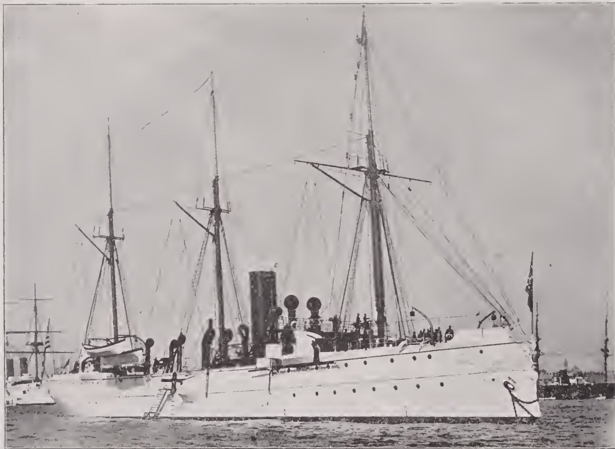
BENNINGTON —Twin-screw, steel, gunboat; 1,710 tons displacement; length, 230 feet; breadth, 36 feet; mean draft, 14 feet; horse power, 3,436; main battery, six 6-inch breech-loading rifles; secondary battery, two 6-pounder and two 3-pounder rapid-fire guns, two 37-millimetre Hotchkiss revolving cannons and two Gatlings; speed, 17.5 knots; crew, 16 officers and 181 men; cost, $553,875 55-
