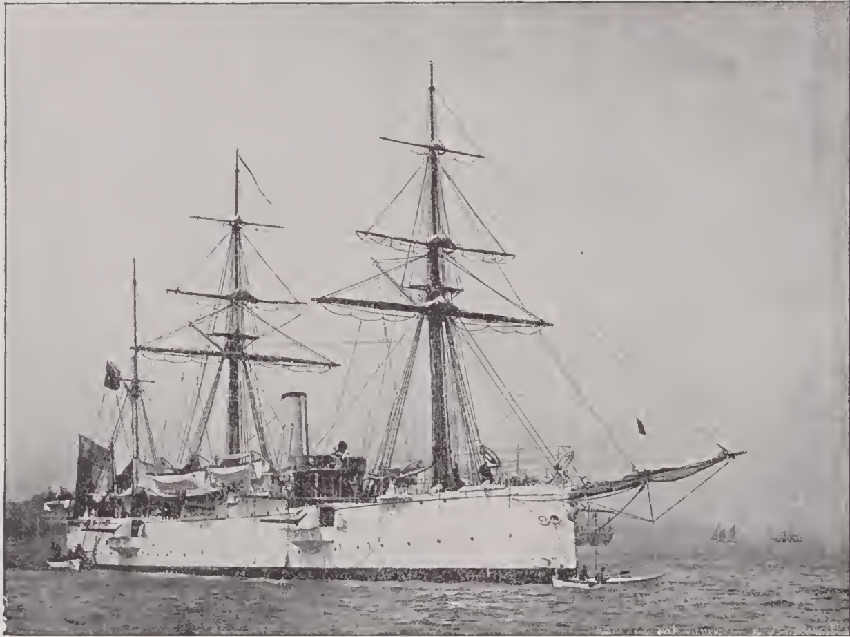
INFANTA ISABEL (Spanish)—Iron cruiser; 1,130 tons displacement; length, 210 feet 11 inches; breadth, 32 feet 2 inches; maximum draft, 12 feet 5 inches; one propeller; horse power, 1,500; batteries, four 4.7-inch (Hontoria guns), two 2.7-inch, three rapid-fire, and four muzzle loading rifled guns; two torpedo tubes; speed, 14 knots an hour; officers and crew, 130.
