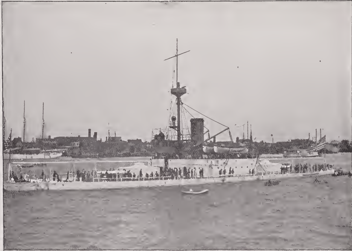
TERROR —Twin-screw, iron, double-turreted monitor; 3,990 tons displacement; length, 250 feet 6 inches; breadth, 55 feet 10 inches; mean draft, 14 feet 6 inches; horse power, 1,600; armor, 7 inches on sides and 11.5 inches on turrets; main battery, four 10-inch breech-loading rifles; secondary battery, two 6-pounder and two 3-pounder rapid-fire guns, two Gatlings and two 37-millimetre Hotchkiss revolving cannons; speed, 12 knots; crew, 15 officers and 136 men; cost, $3,178,046.
