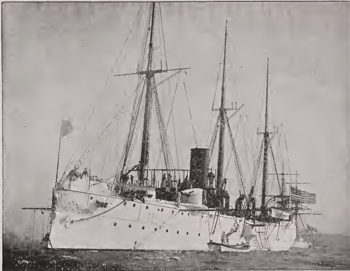
YORKTOWN —Twin-screw, steel, gunboat; 1,710 tons displacement; length, 230 feet; breadth, 36 feet; mean draft, 14 feet; horse power, 3,392; armament, main battery, six 6-inch breech-loading rifles; secondary battery, two 6-pounder and two 3-pounder rapid-fire guns, two 37-millimetre Hotchkiss revolving cannons and two Gatlings; speed, 16.14 knots; crew, 14 officers and 178 men; cost, $455,000.
