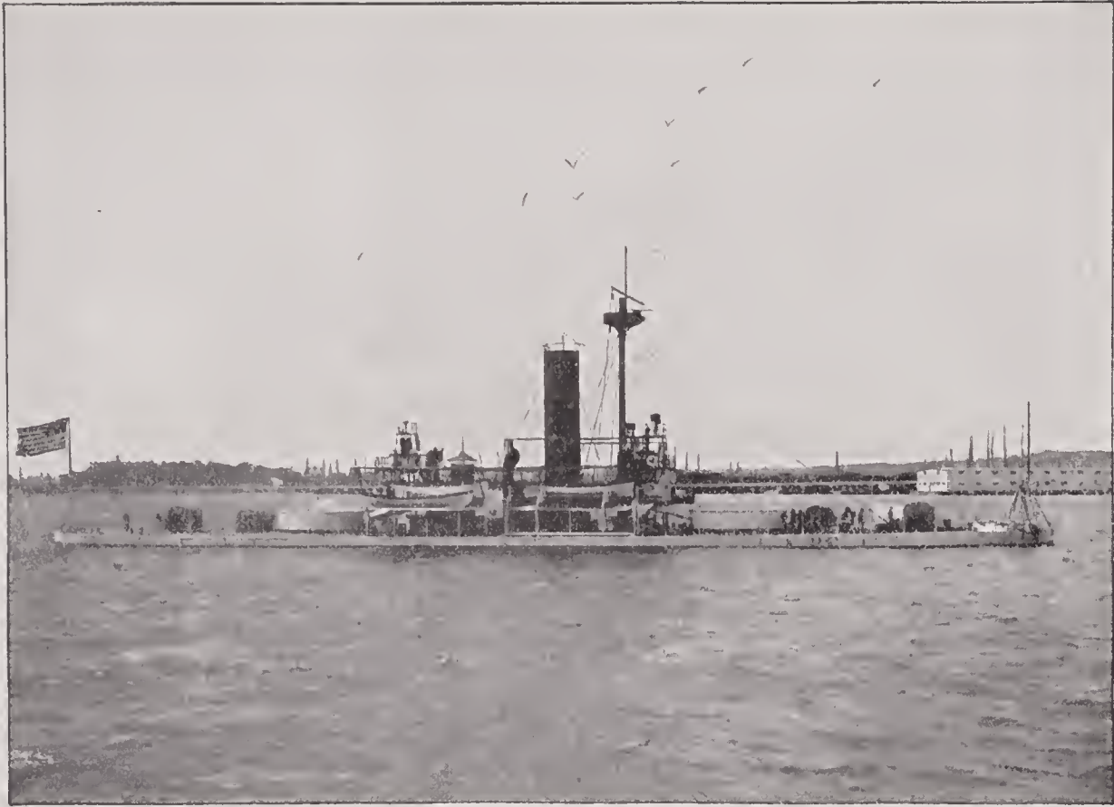
MIANTONOMAH—Twin-screw, iron, double-turreted monitor; 3,990 tons displacement; length, 259 feet 6 inches; breadth, 55 feet 10 inches; mean draft, 14 feet 6 inches; horse power, 1,426; armor, 7 inches on sides and 11.5 inches on turrets; main battery, four 10-inch breech-loading rifles; secondary battery, two 6-pounder and two 3-pounder rapid-fire guns, and two 1-pounder rapid-fire cannons; speed, 10.5 knots; crew, 13 officers and 136 men; cost, $3,178,046.
