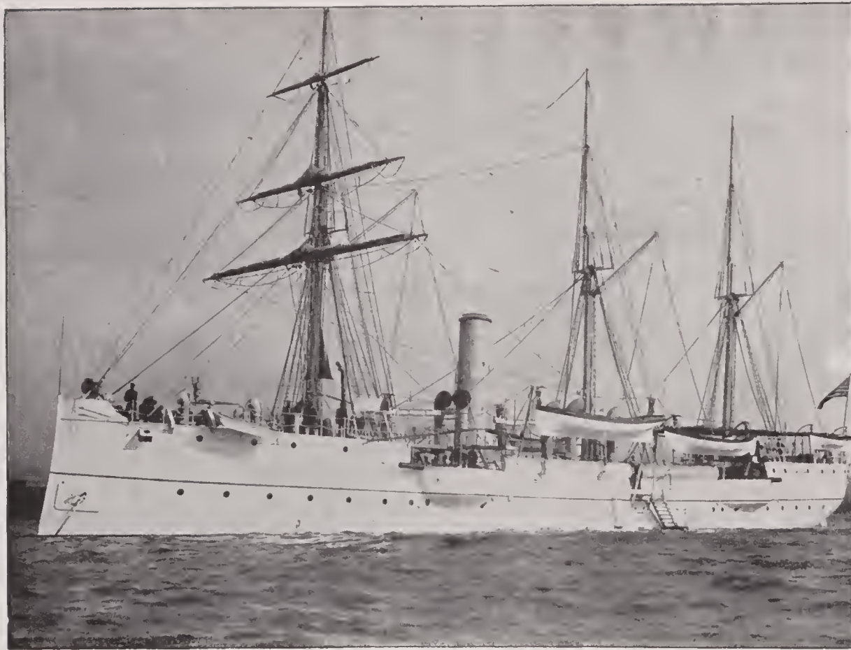
PETREL —Single screw, steel, gunboat; 892 tons displacement; length, 176 feet; breadth, 31 feet; mean draft, 11 feet 7 inches; horse power, 1,095; armament, main battery, four 6-inch breech-loading rifles; secondary battery, one 1-pounder rapid-fire gun, two 37-millimetre Hotchkiss revolving cannons and two Gatlings; speed, 11.7 knots; crew, 10 officers and 122 men; cost, $307,966.55. In the engagement with the Spanish fleet at Manila, May 1, 1898.
