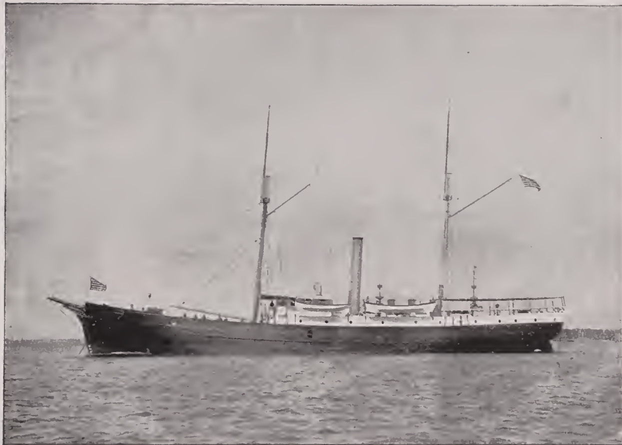
FERN —Single screw, wooden, transport steamer; 1,840 tons displacement. This vessel is used at the North Atlantic station. At present it is attached to the squadron in Cuban waters.
