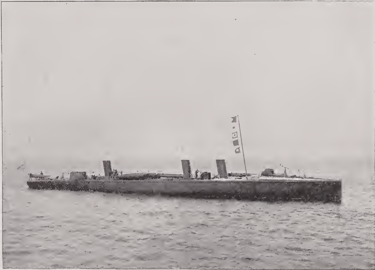
PORTER —Twin-screw, steel, torpedo boat; 180 tons displacement; length, 175 feet 9 inches; breadth, 17 feet; mean draft, 5 feet 6 inches; armament, four 1-pounder rapid-fire guns and three 18-inch Whitehead torpedo tubes; speed, 27.5 knots an hour; crew, 4 officers and 16 men; cost, $147,000. The normal coal supply is nine tons.
