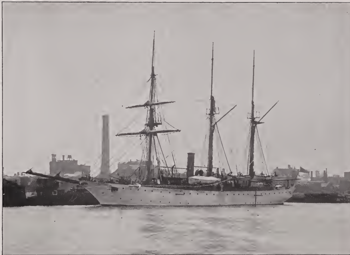
ANNAPOLIS —Single screw, composite gunboat; 1,000 tons displacement; length, 168 feet; breadth, 36 feet; mean draft, 12 feet; horse power, 1,227; main battery, six 4-inch rapid-fire guns; secondary battery, four 6-pounder and two 1-pounder rapid-fire guns; speed, 12 knots; crew, 11 officers and 135 men; cost, $230,000.
