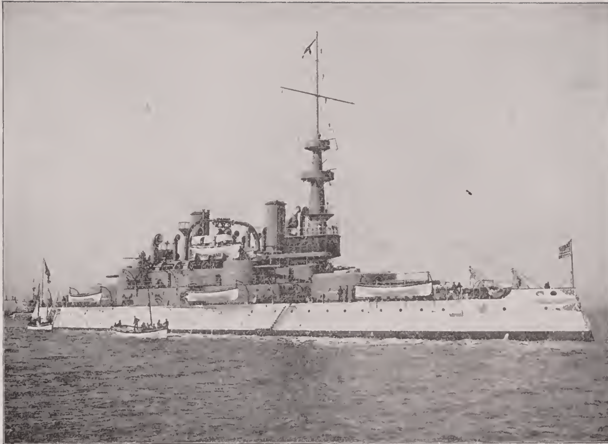
INDIANA —First class, twin-screw, steel battleship; 10,288 tons displacement; length, 348 feet; breadth, 69 feet 3 inches; mean draft, 24 feet; horse power, 9,738; armor, 18 inches on the sides, from 6—15 inches on the turrets, and from 6—17 inches on the barbets; main battery, four 13-inch, eight 8-inch, and four 6-inch breach-loading rifles; secondary battery, 30 rapid-fire guns of small calibre; speed, 15.547 knots; crew, 38 officers and 438 men; cost, $3,020,000.
