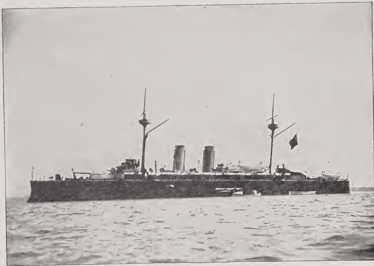
VIZCAYA (Spanish)—Iron, barbette, armored cruiser; 7,000 tons displacement; length, 340 feet; breadth, 65 feet; maximum draft, 21 feet 6 inches; horse power, 13,000; armor, belt 12 inch, gun positions 10½ inch, deck plating 3 inch; batteries, two 11-inch, ten 5.5-inch rapid-fire, two 2.7-inch, eight 12.2-inch, four 1.4-inch, and two muzzle loading rifled guns; six torpedo tubes; speed, 20 knots; officers and crew, 500; cost, $600,000.
