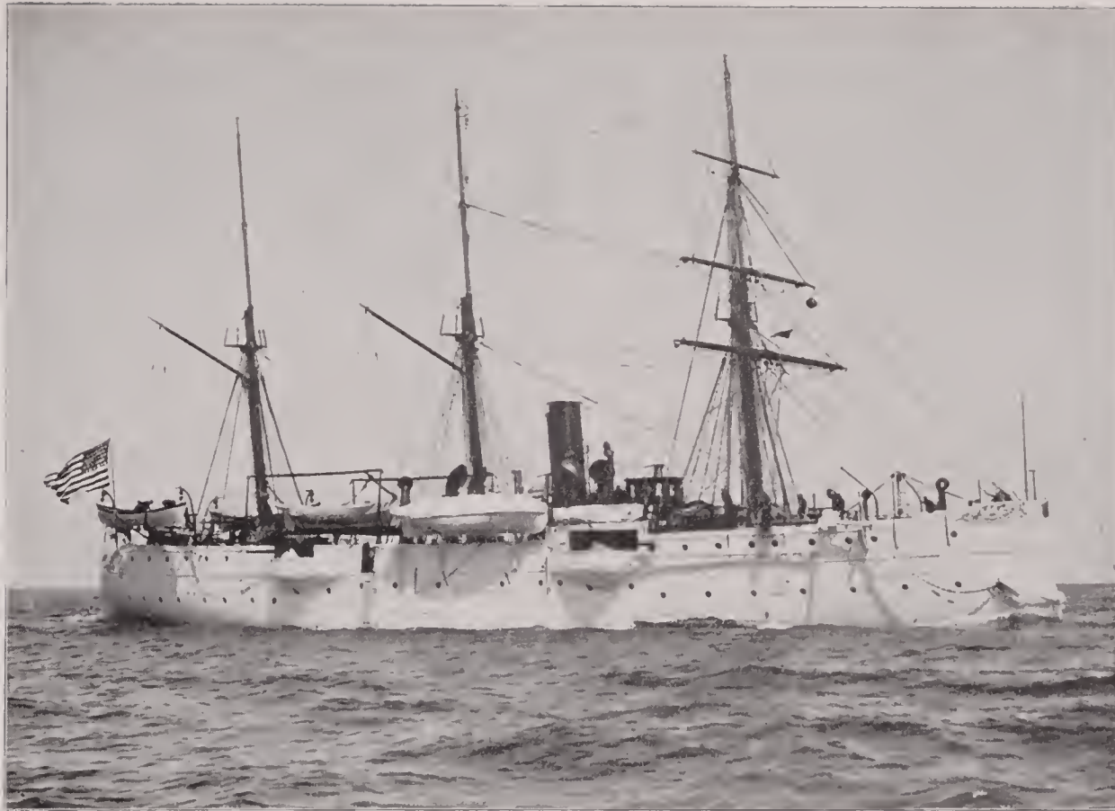
BANCROFT —Twin-screw, steel, gunboat; 832 tons displacement; length, 187 feet 6 inches; breadth, 32 feet; mean draft, 11 feet 6 inches; horse power, 1,213; main battery, four 4-inch rapid-fire guns; secondary battery, two 6-pounder and two 3-pounder rapid-fire guns, one 1-pounder rapid-fire cannon, one 37-millimetre Hotchkiss revolving cannon and one Gatling; speed, 14.3 knots; crew, 10 officers and 120 men; cost, $297,360.17. This is a practice vessel for naval cadets.
