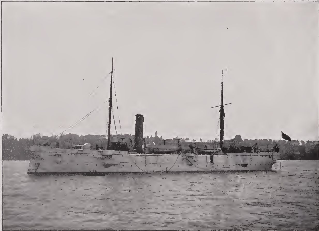
MACHIAS —Twin-screw, steel, gunboat; 1,177 tons displacement; length, 204 feet; breadth, 32 feet; mean draft, 12 feet; horse power, 2,046; main battery, eight 4-inch rapid-fire guns; secondary battery, four 6-pounder and two 1-pounder rapid-fire guns; speed, 15.4 knots; crew, 11 officers and 143 men; cost, $318,500.
