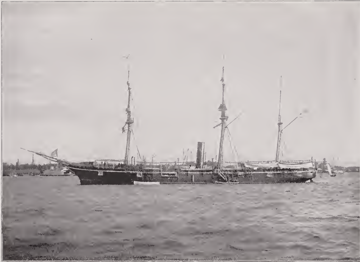
YANTIC —Single screw, wooden, cruiser; 900 tons displacement; length, 179 feet 6 inches; breadth, 30 feet; horse power, 310; main battery, two 9-inch smooth-bore guns, one 8-inch muzzle-loading rifle and one 60-pounder rifle; secondary battery, one 12-pounder rapid-fire gun, one 3-pounder breech-loading Howitzer and one Gatling; speed, 8.3 knots; cost, $206,262.93. The keel of this old navy vessel was laid in 1862.
