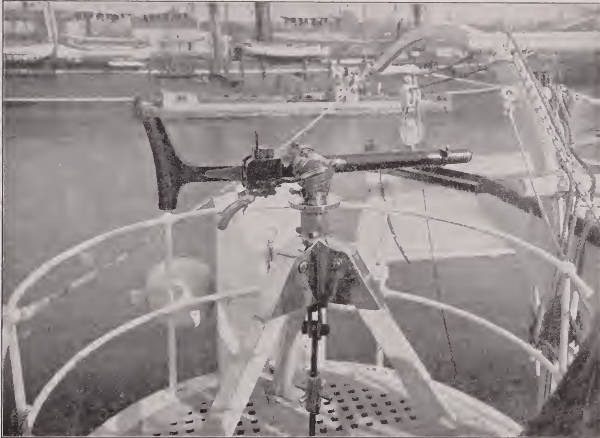
HOTCHKISS RAPID-FIRE GUN —The 1-pounder Hotchkiss rapid-fire gun is made of all steel. Weight, 120 pounds; total length, 62 inches; greatest diameter of gun body, 4.72 inches; weight of cartridge complete, 1.5 pounds; weight of shell, 1 pound; weight of charge, 2.8 ounces; initial velocity, 1,319 feet; range at 40 degrees elevation, 2\frac{1}{8} miles. It is composed of a central tube, jacket and locking ring. The twist of rifling is uniform; angle of rifling, 6 degrees; and the number of grooves is twelve.
