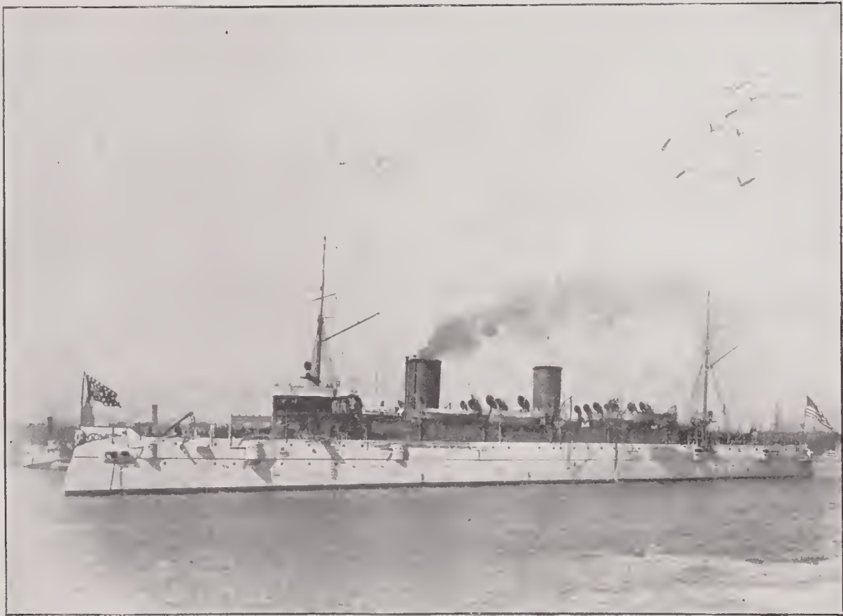
MINNEAPOLIS —Triple-screw, steel, protected cruiser; 7,375 tons displacement; length, 411 feet 7 inches; breadth, 58 feet 2 inches; mean draft, 22 feet 6 inches; horse power, 20,862; main battery, one 8-inch breech-loading rifle, two 6-inch and eight 4-inch rapid-fire guns; secondary battery, twelve 6-pounder and four 1-pounder rapid-fire guns, and four Gatlings; speed, 23.7 knots an hour; crew, 38 officers and 656 men; cost, $2,690,000.
