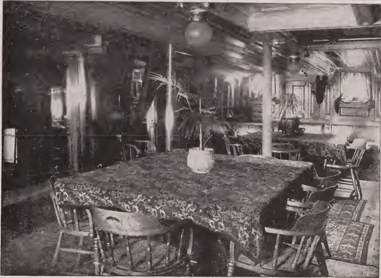
WARD-ROOM ON THE CRUISER CHICAGO —A ward-room is an apartment on the after end of the lower gun deck of a ship of war, usually occupied as a mess-room by the commissioned officers, except the captain.
