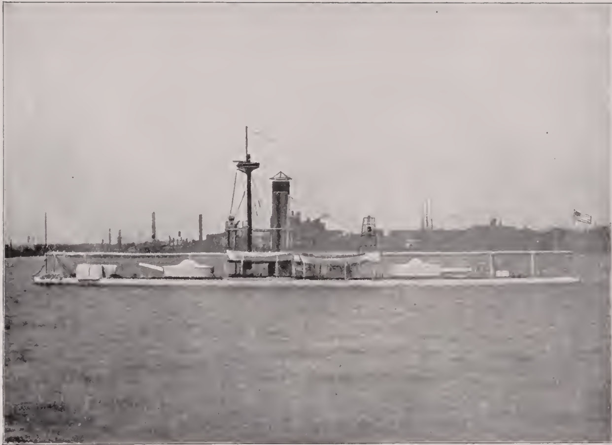
MONADNOCK —Twin-screw, iron, double-turreted monitor; 3,990 tons displacement; length, 259 feet 6 inches; breadth, 55 feet 10 inches; mean draft, 14 feet 6 inches; horse power, 3,000; armor, 9 inches on sides, 7.5 inches on turrets and 11.5 inches on barbettes; main battery, four 10-inch breech-loading rifles and two 4-inch rapid-fire guns; secondary battery, two 6-pounder and two 3-pounder rapid-fire guns, two 37-millimetre Hotchkiss revolving cannons, and two 1-pounder rapid-fire cannons; speed, 14.5 knots; crew, 26 officers and 145 men; cost, $3,178,046.
