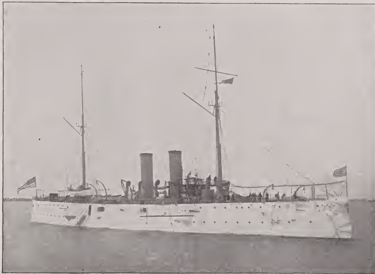
CINCINNATI —Twin-screw, steel, protected cruiser; 3,183 tons displacement; length, 300 feet; breadth, 42 feet; mean draft, 18 feet; horse power, 10,000; main battery, ten 5-inch and one 6-inch rapid-fire guns; secondary battery, eight 6-pounder rapid-fire guns, two 1-pounder rapid-fire cannons and two Gatlings; speed, 19 knots; crew, 20 officers and 292 men; cost, $1,100,000.
