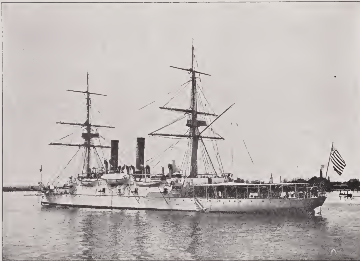
BOSTON —Single screw, steel, protected cruiser; 3,189 tons displacement; length, 270 feet 3 inches; breadth, 42 feet; mean draft, 17 feet; horse power, 4,030; main battery, six 6-inch and two 8-inch breech-loading rifles; secondary battery, two 6-pounder and two 3-pounder rapid-fire guns, two 1-pounder rapid-fire cannons, two 47-millimetre Hotchkiss revolving cannons and two Gatlings; speed, 15.6 knots; crew, 19 officers and 205 men; cost, $809,923.44. With Admiral Dewey's fleet in the destruction of the Spaniards at Manila, May 1, 1898.
