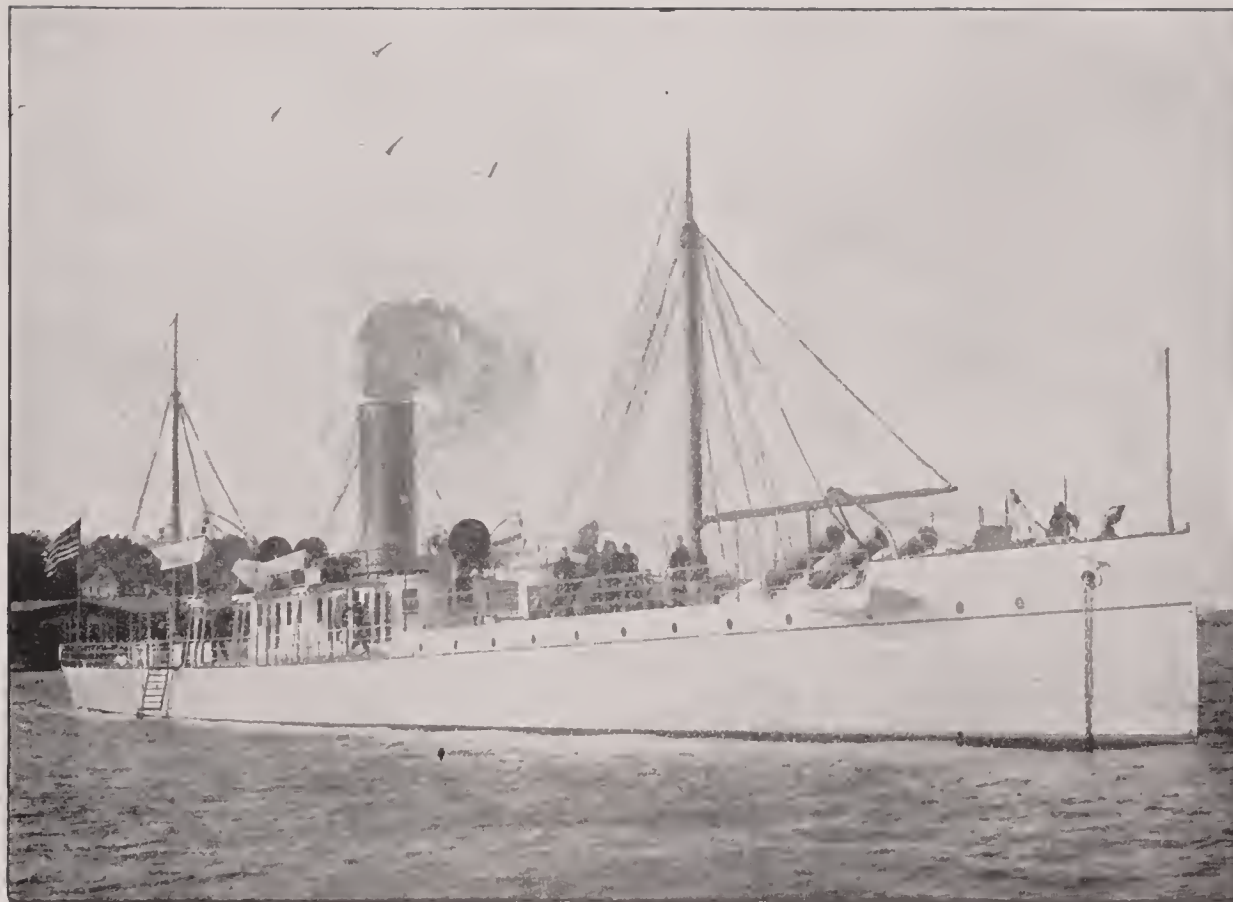
VESUVIUS —Twin-screw, steel, dynamite gun vessel; 929 tons displacement; length, 252 feet; breadth, 26 feet 6 inches; mean draft, 10 feet 1 inch; horse power, 3,796; armament, main battery, three 15-inch dynamite guns; secondary battery, three 3-pounder rapid-fire guns; speed, 21.4 knots; crew, 6 officers and 64 men; cost, $350,000.
