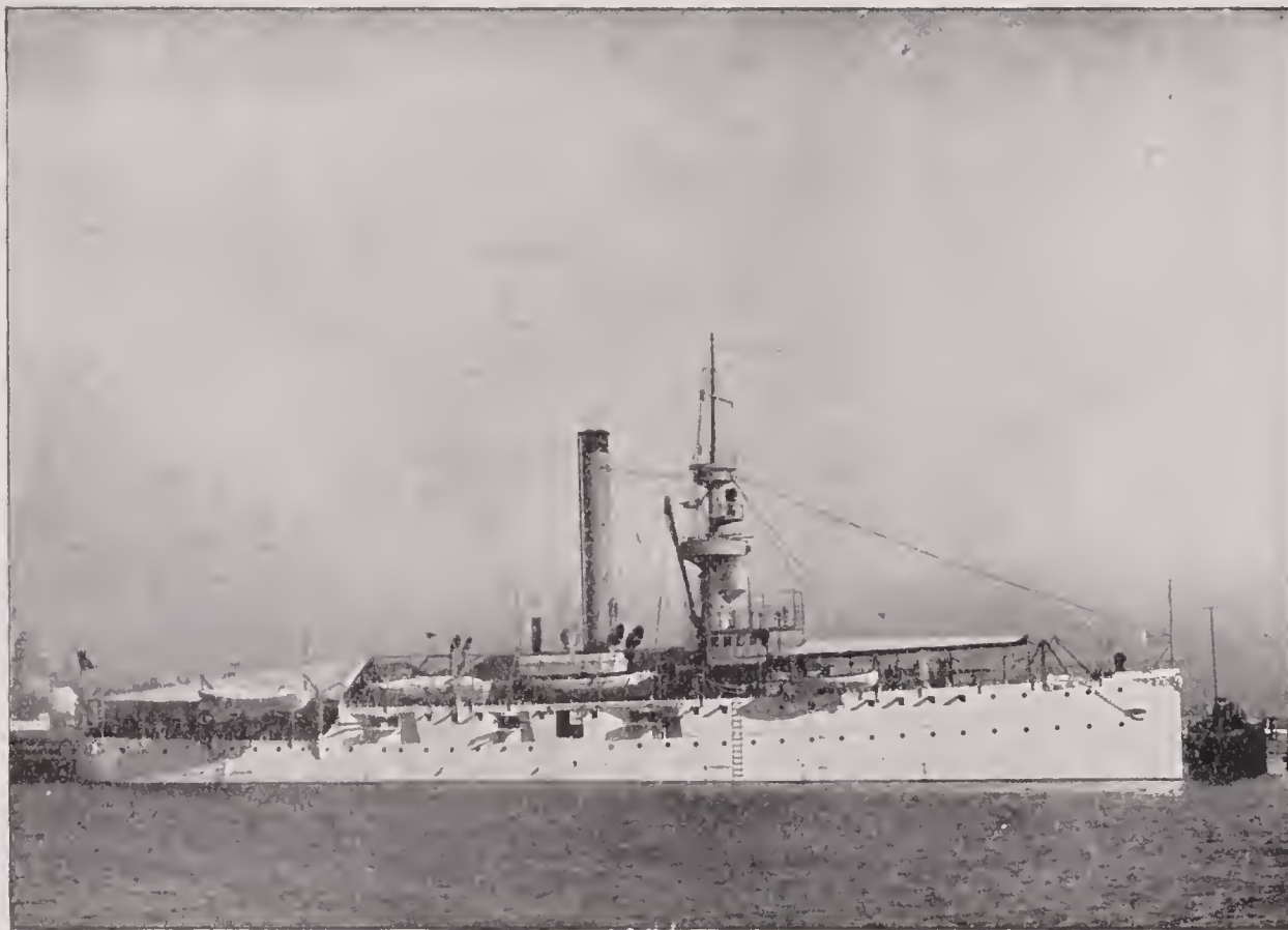
HELENA —Twin-screw, steel, light draft gunboat; 1,392 tons displacement; length, 250 feet 9 inches; breadth, 40 feet 1 \frac{3}{8} inches; mean draft, 9 feet; horse power, 1,600; armament, main battery, eight 4-inch rapid-fire guns; secondary battery, four 6-pounder and four 1-pounder rapid-fire guns and two Gatlings; speed, 13 knots; crew, 10 officers and 160 men; cost, $280,000.
