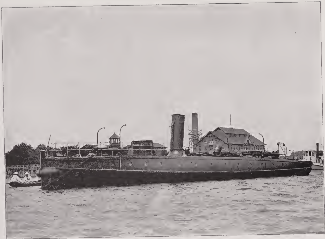
STILETTO —Single screw, wooden, torpedo boat; 31 tons displacement; length, 88 feet 6 inches; breadth, 11 feet; mean draft, 3 feet; horse power, 359; armament, six rapid-fire guns of small calibre; speed, 18.2 knots an hour; crew, 1 officer and 5 men; cost, $25,000. The smallest vessel of this class in the United States navy.
