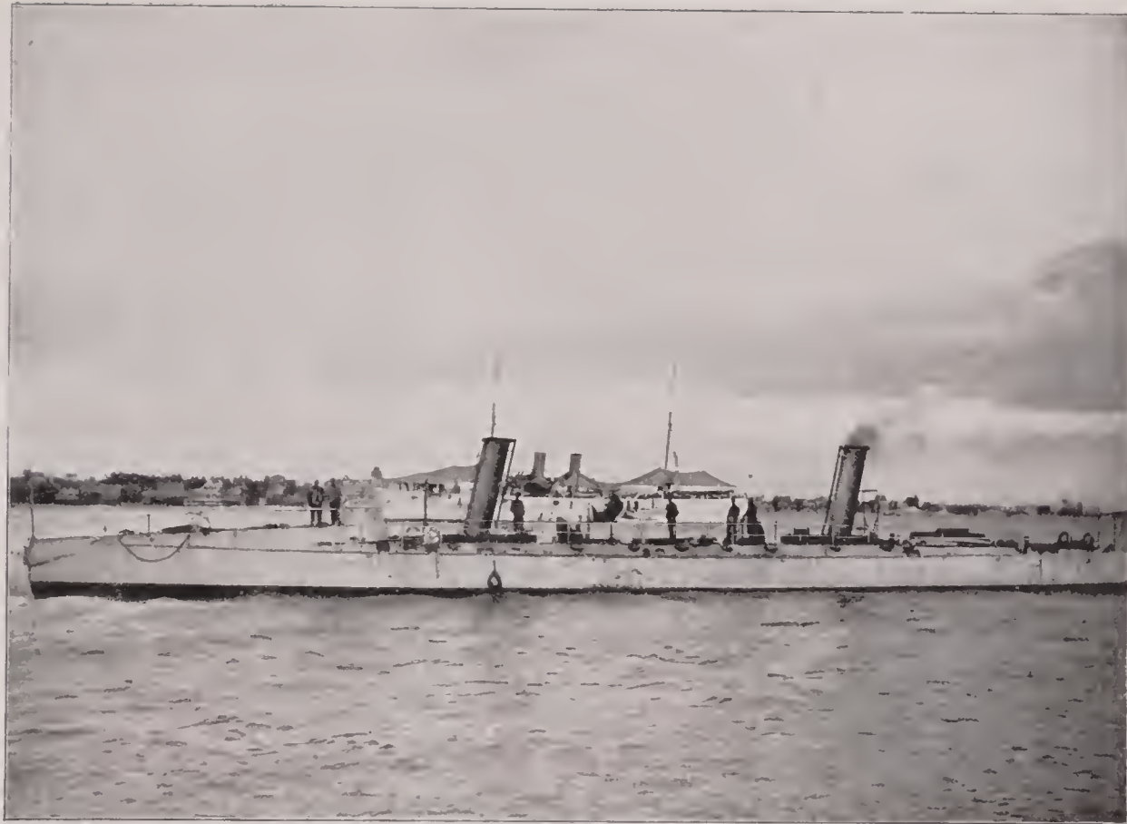
ERICSSON --Twin-screw, steel, torpedo boat; 120 tons displacement; length, 149 feet; breadth, 15 feet 6 inches; mean draft, 4 feet 9 inches; horse power, 1,800; batteries, three 1-pounder rapid-fire guns and three 18-inch Whitehead torpedo tubes; speed, 24 knots; crew, 3 officers and 20 men; cost, $113,500.
