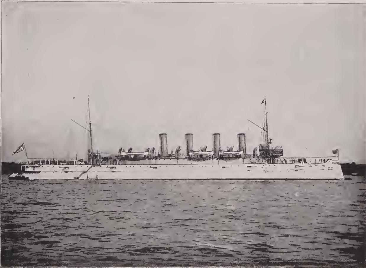
COLUMBIA —Triple-screw, steel, protected cruiser; 7,375 tons displacement; length, 411 feet 7 inches; breadth, 58 feet 5 inches; mean draft, 22 feet 6 inches; horse power, 18,509; armament, main battery, two 6-inch and eight 4-inch rapid-fire guns, and one 8-inch breech-loading rifle; secondary battery, twelve 6-pounder rapid-fire guns, four 1-pounder rapid-fire cannons, and four Gatlings; speed, 22.8 knots an hour; crew, 40 officers and 429 men; cost, $2,725,000.
