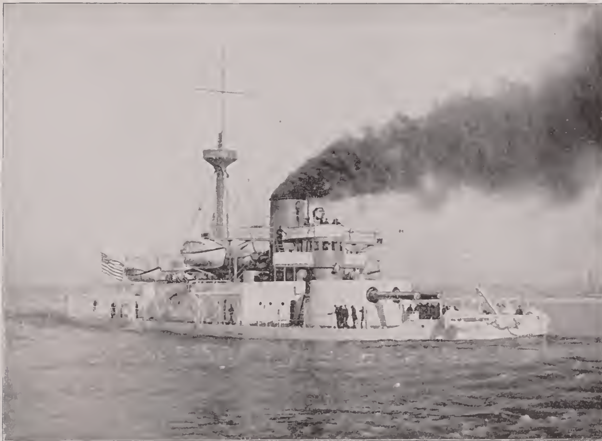
PURITAN —Twin-screw, iron, double turret monitor for coast defense; 6,060 tons displacement; length, 289 feet 6 inches; breadth, 60 feet 1½ inches; mean draft, 18 feet; horse power, 3,700; armor, 14 inches on the sides, 8 inches on the turrets, and 14 inches on the barbets; main battery, four 12-inch breech-loading rifles and two 4-inch rapid-fire guns; secondary battery, six 6-pounder rapid-fire guns, four Gatlings and two 37-millimetre Hotchkiss revolving cannons; speed, 12.4 knots; crew, 22 officers and 208 men; cost, $3,178,046.
