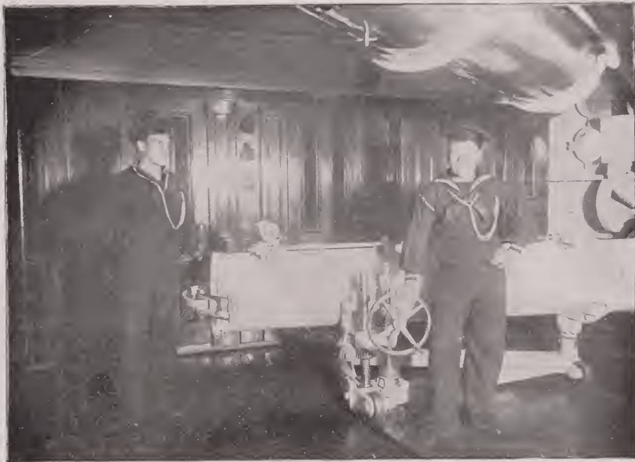
TORPEDO GUN ON THE MAINE —The Maine carried four torpedo tubes, or what are sometimes spoken of as torpedo guns. The explosive with which a torpedo is charged is fired in one of three distinct ways: by contact, by concussion, or by electricity. Nearly every year the torpedo is being made more deadly, and, with very few exceptions, all the United States battleships carry from one to six tubes.
