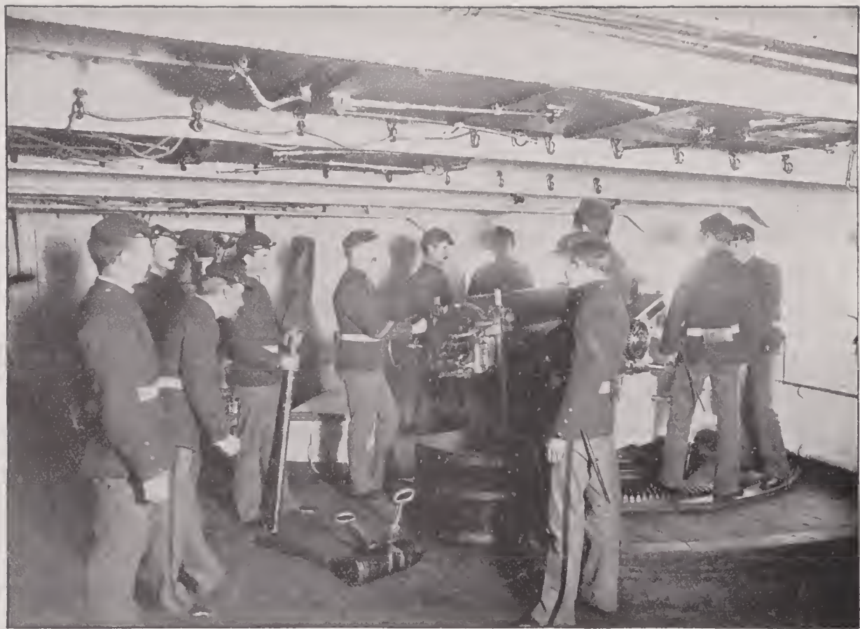
EIGHT-INCH RIFLE PRACTICE —Everything is ready for the marksman, whose sign is awaited with silent attention. As soon as he has satisfied himself that all is well, he either motions with his hand or speaks the word that sends the 250-pound projectile to its destination. The shell of an 8-inch breech-loading rifle will perforate steel of 15.51 inches thickness at the muzzle, and 12.36 inches thick at 1,500 yards.
