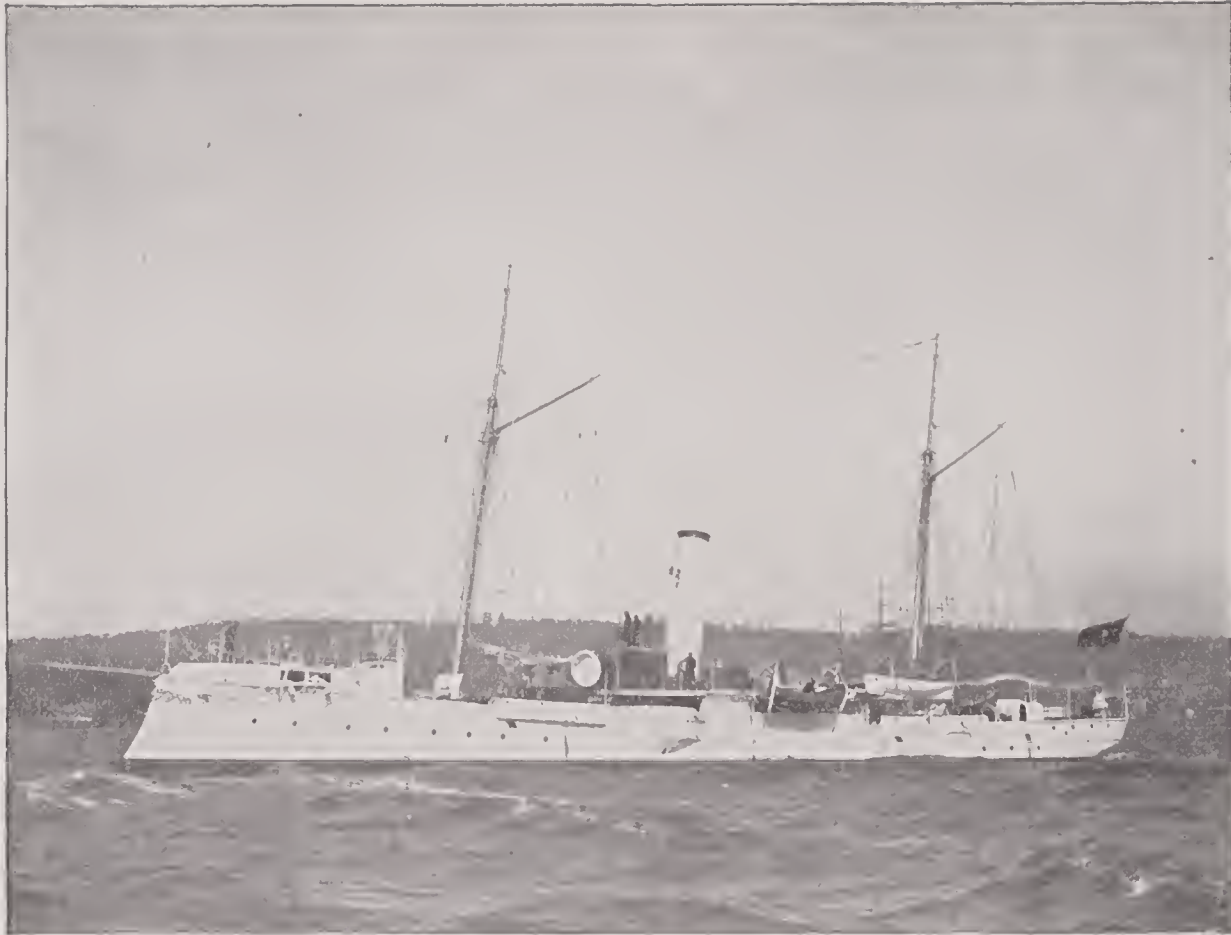
NUEVA ESPANA (Spanish)—Steel cruiser; 630 tons displacement; length, 190 feet; breadth, 23 feet; maximum draft, 11 feet 9 inches; two propellers; horse power, 2,600; batteries, two 4.7-inch (Hontoria) and four 2.2-inch rapid-fire guns with one muzzle loading rifled gun; two torpedo tubes; speed, 18 knots an hour; officers and crew, 91.
