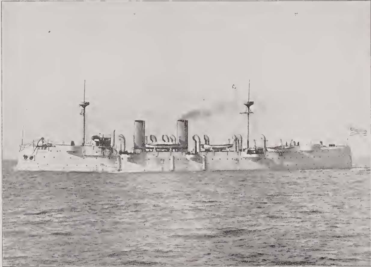
BALTIMORE —Twin-screw, steel, protected cruiser; 4,600 tons displacement; length, 327 feet 6 inches; breadth, 48 feet 6 inches; mean draft, 19 feet 7 inches; horse power, 10,064; main battery, four 8-inch and six 6-inch breech-loading rifles; secondary battery, four 6-pounder and two 3-pounder rapid-fire guns, two 1-pounder rapid-fire cannons, four 37-millimetre Hotchkiss revolving cannons and two Gatlings; speed, 20.09 knots; crew, 36 officers and 350 men; cost, $1,426,504.93. With Admiral Dewey's fleet in the fight with the Spaniards at Manila, May 1, 1898.
