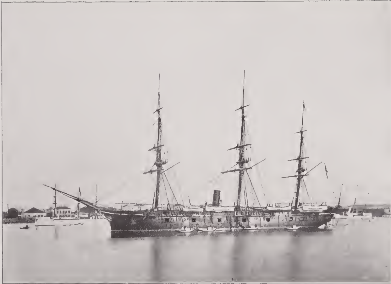
LANCASTER —Single screw, wooden cruiser; 3,290 tons displacement; length, 235 feet 8 inches; breadth, 46 feet; horse power, 733; speed, 9.6 knots; main battery, 12 guns. This is one of the old navy vessels, the keel having been laid in 1857. Cost, $668,769.
