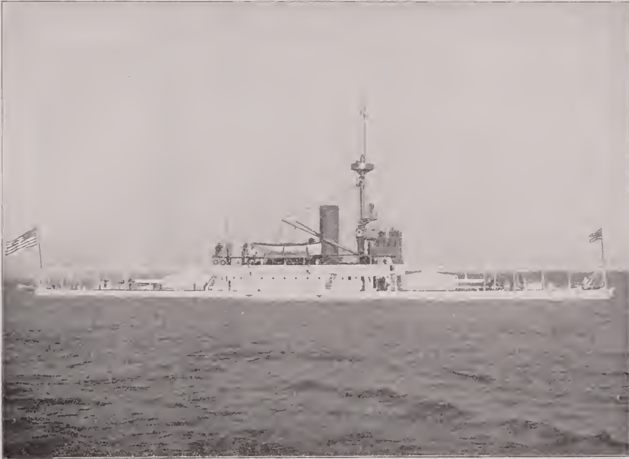
AMPHITRITE —Twin-screw, iron, double-turreted monitor; 3,990 tons displacement; length, 259 feet 6 inches; breadth, 55 feet 10 inches; mean draft, 14 feet 6 inches; horse power, 1,600; armor, 9 inches on sides, 7.5 inches on turrets and 11.5 inches on barbets; main battery, four 10-inch breech-loading rifles and two 4-inch rapid-fire guns; secondary battery, two 6-pounder and two 3-pounder rapid-fire guns, two 37-millimetre Hotchkiss revolving cannons, and two 1-pounder rapid-fire cannons; speed, 12 knots; crew, 26 officers and 145 men; cost, $3,178,046.
