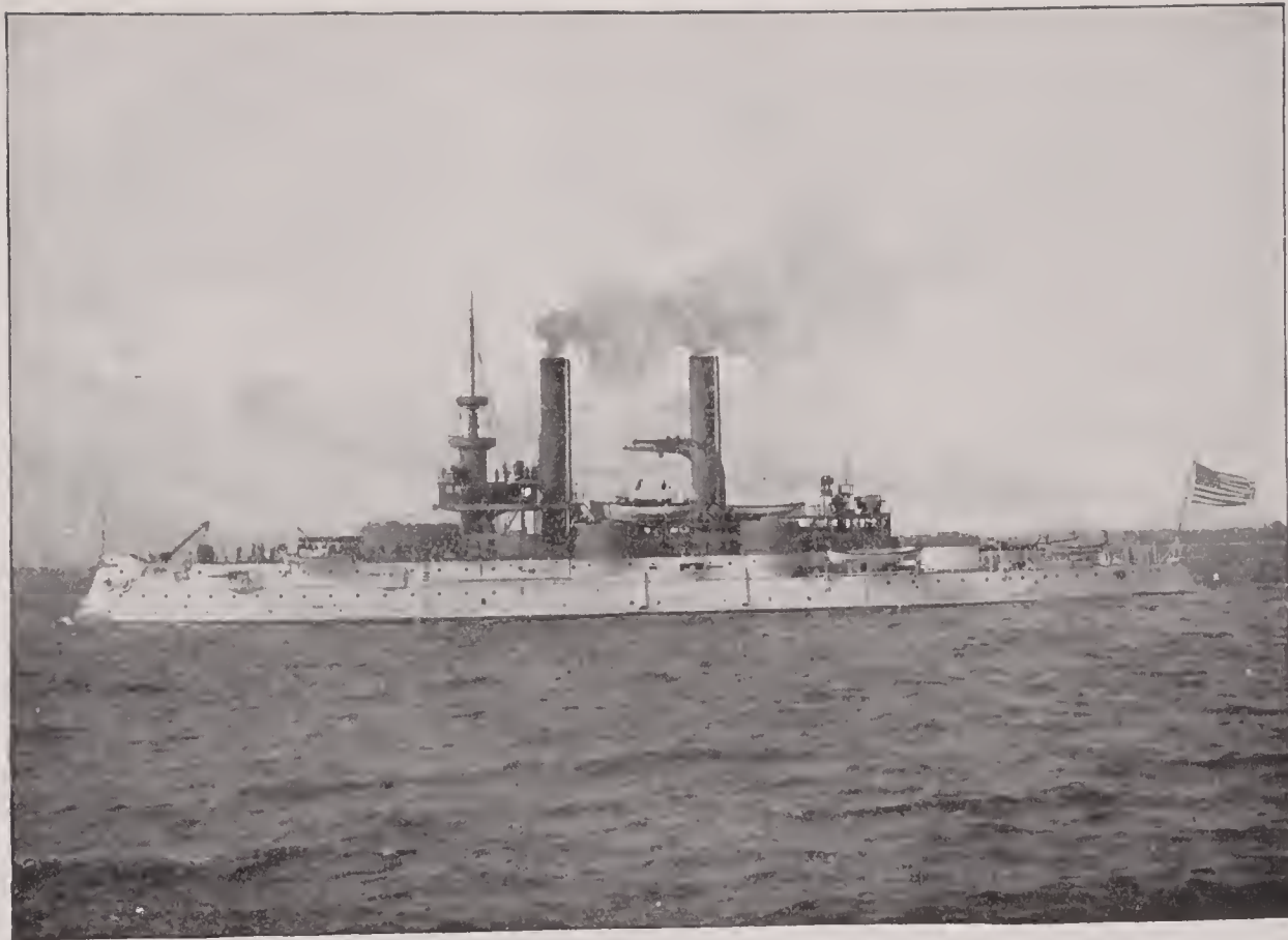
IOWA —First class, twin-screw, steel battleship; 11,296 tons displacement; length, 360 feet; breadth, 72 feet 2½ inches; mean draft, 24 feet; horse power, 12,105; armor, 14 inches on the sides, from 5½—15 inches on the turrets, and from 6—15 inches on the barbets; main battery, four 12-inch, eight 8-inch, and six 4-inch rapid-fire guns; secondary battery, twenty 6-pounder and four 1-pounder rapid-fire guns and four Gatlings; speed, 17.087 knots; crew, 36 officers and 469 men; cost, $3,010,000.
