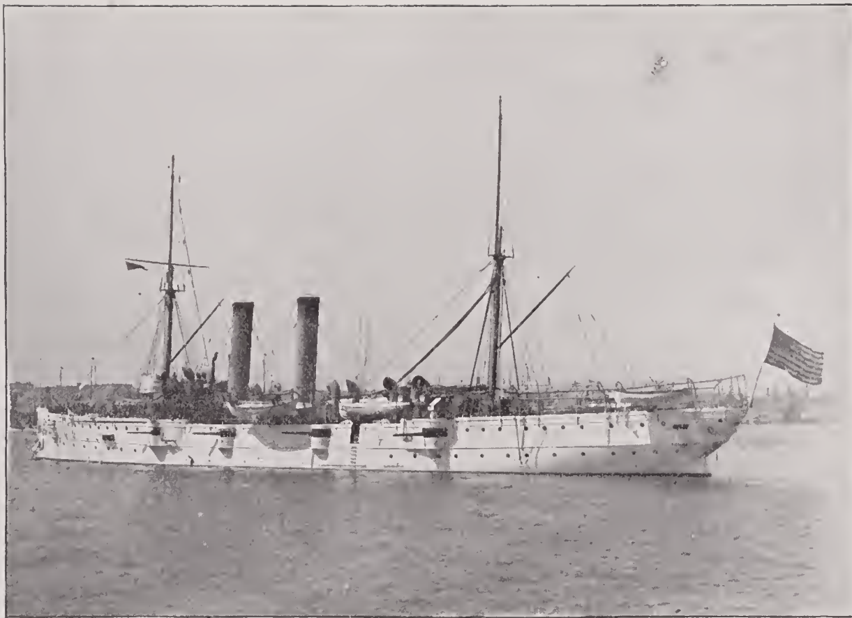
MONTGOMERY —Twin-screw, steel, unprotected cruiser; 2,079 tons displacement; length, 257 feet; breadth, 37 feet; mean draft, 14 feet 6 \frac{1}{4} inches; horse power, 5,580; main battery, nine 5-inch rapid-fire guns; secondary battery, six 6-pounder rapid-fire guns, two 1-pounder rapid-fire cannons and two Gatlings; speed, 19.5 knots; crew, 20 officers and 254 men; cost, $612,500.
