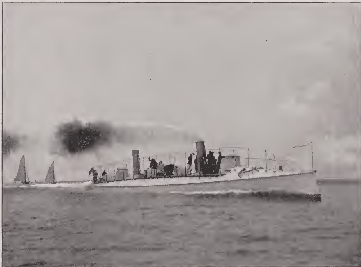
CUSHING —Twin-screw, steel, torpedo boat; 105 tons displacement; length, 139 feet; breadth, 14 feet 3 inches; mean draft, 4 feet 11 inches; horse power, 1,720; armament, three 1-pounder rapid-fire guns and three 18-inch Whitehead torpedo tubes; speed, 22.5 knots; crew, 3 officers and 20 men; cost, $82,750.
