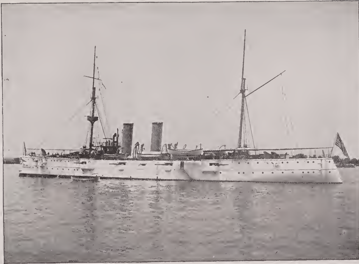
RALEIGH —Twin-screw, steel, protected cruiser; 3,213 tons displacement; length, 300 feet; breadth, 42 feet; mean draft, 18 inches; horse power, 10,000; main battery, ten 5-inch and one 6-inch rapid-fire guns; secondary battery, eight 6-pounder rapid-fire guns, four 1-pounder rapid-fire cannons and two Gatlings; speed, 19 knots; crew, 20 officers and 292 men; cost, $1,100,000. With Admiral Dewey in the annihilation of the Spanish fleet at Manila, May 1, 1898.
