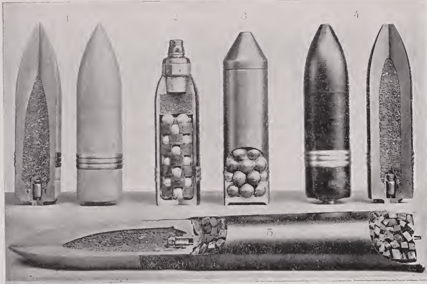
RAPID-FIRE AMMUNITION —The rapid-fire gun ammunition is here presented in sections which show the inner construction of the shells and their contents. The cartridge cases are composed of brass or copper and known as metallic ammunition. No. 5, lying lengthwise, shows the construction of a cartridge with a total weight of 96 pounds. The solid brass case weighs 18 pounds; the steel shell, 50 pounds, and the powder charge is 28 pounds. Then there are the cap and fuse.
