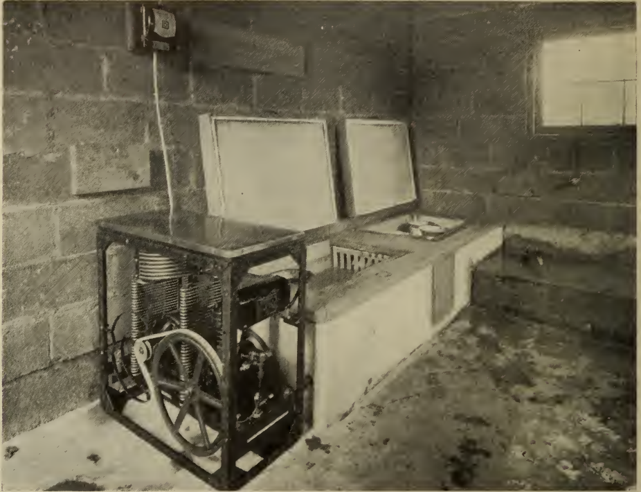
Fig. 4—Cooling milk by mechanical refrigeration in an insulated cooling tank.
