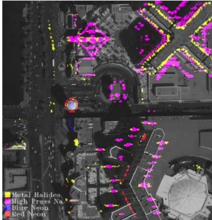
Figure 15. Classification of night lighting for selected lighting types using binary encoding. Classification map overlain on Quickbird image to illustrate building association with lighting type (From Kruse & Elvidge 2011).
