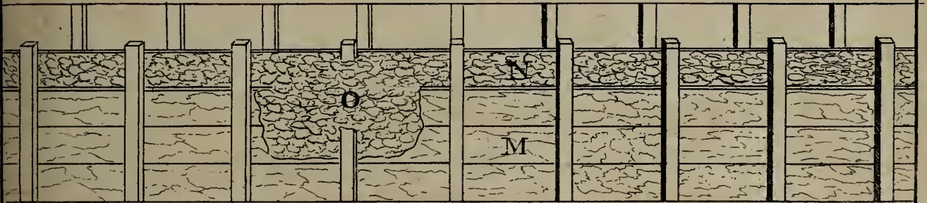
M. Planks laid edgeway. N. Inward part of the Wall. O. Face of the Wall the Planks being taken away.
