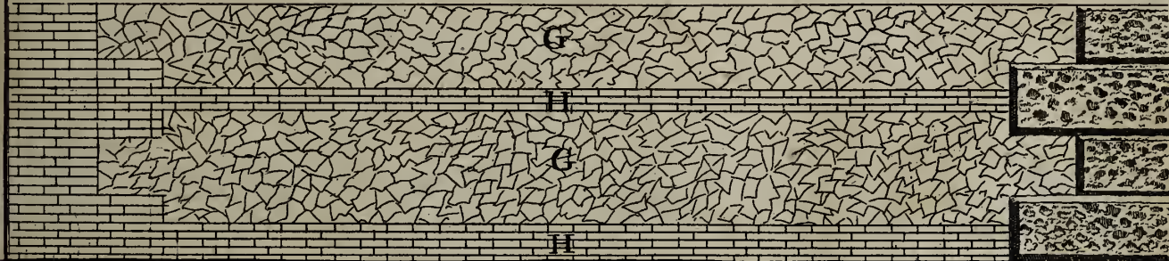
G. Cement or River Pebbles. H. Courses of Bricks y t bind y e whole Wall
