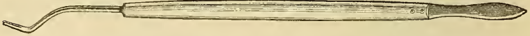
McAdams's combined spatula and stopper, constructed of hard platina and mounted in ivory, suitable for oxychloride and pyrophosphate of zinc fillings.
