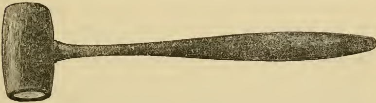
Hand mallet, the head of which is constructed of hard wood filled with lead, which lessens the amount of vibration when used.
