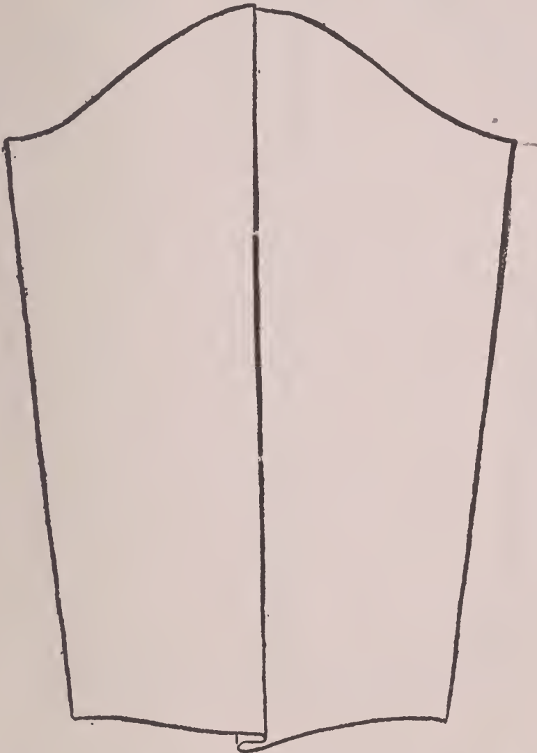
Fig. (86) A sleeve pattern folded to take out the fullness at the bottom
