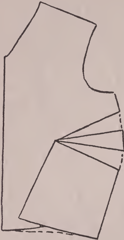
Fig. (101) Pleats at the sides will help to take out the fullness at the bottom of a waist
