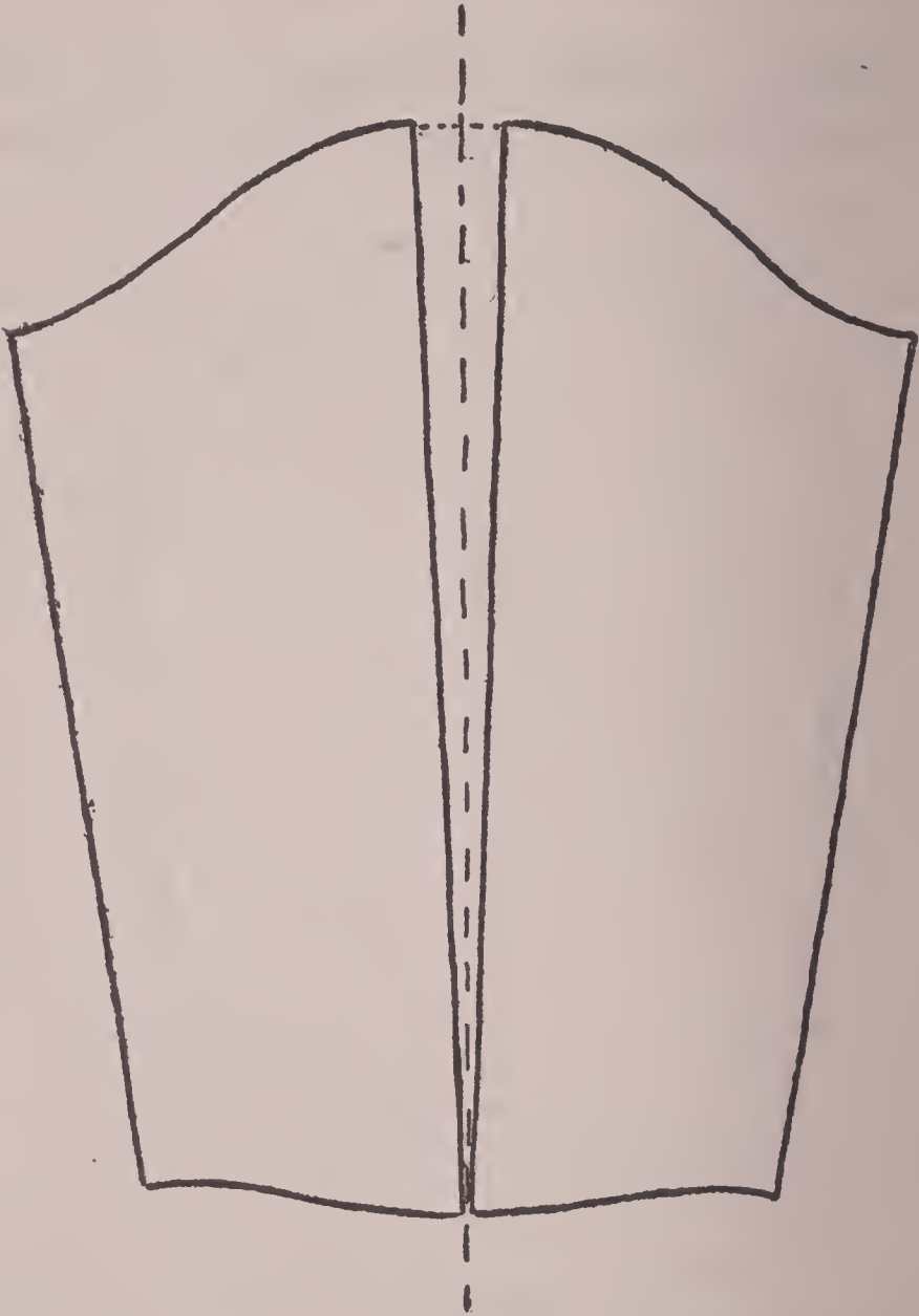
Fig. (87) Spreading a sleeve pattern at the top to make it larger
