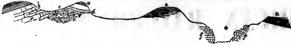
a, a, Sandstone; b, Gneiss; c, Serpentine; d, Adit in the Parish Bed; e, Excavation at the Kearney Bed; f, f, Ore.
