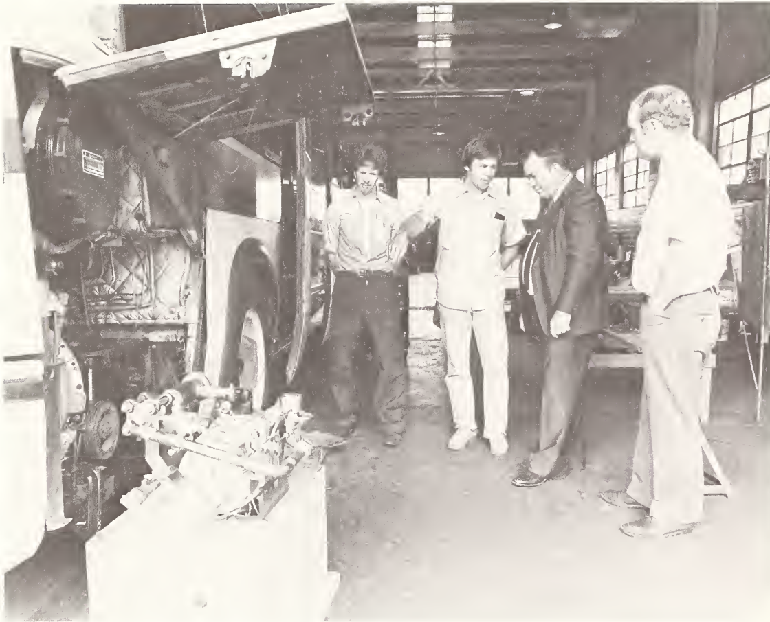
This rotary screw compressor is being tested on bus air conditioning systems in San Antonio to improve efficiency and lower operating costs.
