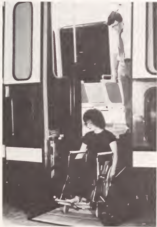
This pre-revenue service test of a wheel-chair lift at MUNI resulted from an UMTA-sponsored study on the feasibility of lift retrofits.
