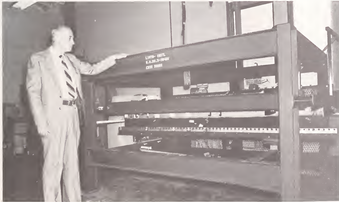
This test stand is used for evaluating both the propulsion and levitation properties of linear induction motors.
