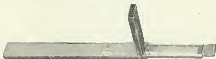
Figure 2 shows the instrument open ready for use. The cap is removed, the wire at the end of the cap is slipped over the end of the instrument to make a shield for the observer's eye.
