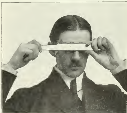
Figure 3 shows the position in which the photometer is held when in use, resting firmly on the nose, with the hole in the case before the eye.
