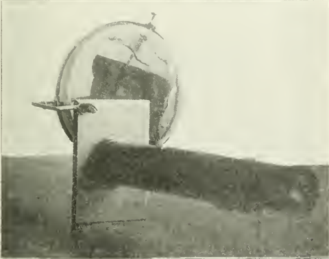
Fig. 3.—View of a hand microscope with the Petri-dish-glycerin-jelly preparation fastened in a special device and so placed as to afford a naked-eye view of the gross preparation. A mounted microscope section of it is seen at one side.
