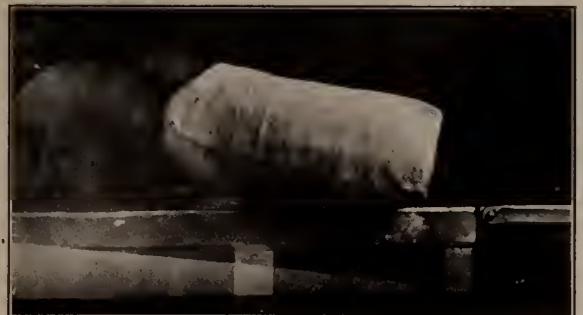
Cast completed showing method of trimming the top. Note the position of the sheet iron strip.
