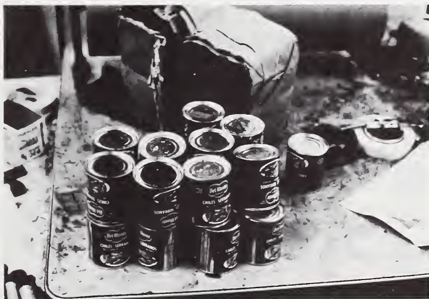
Figure B-2 . Canned food packaged without separators, hammered their way out of the parcel.
