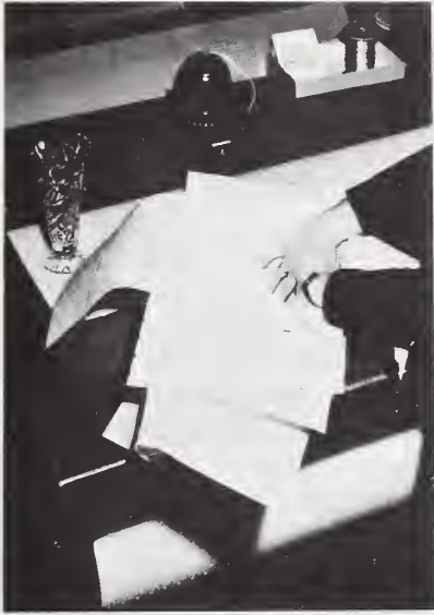
(a) Container is lined with polypropylene foam sheets.
