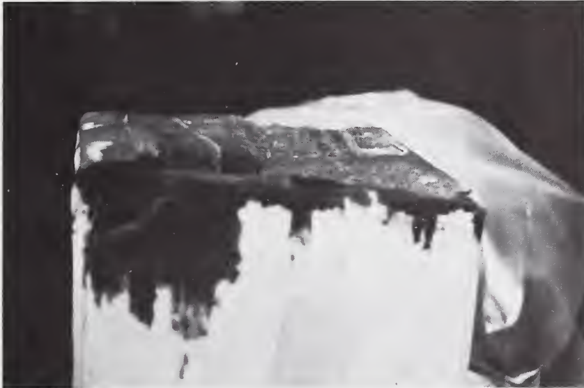
Figure 9. Damaged parcel containing one-gallon can of chocolate syrup. The can had a pry-up lid without a positive mechanical lock. (NBS)
