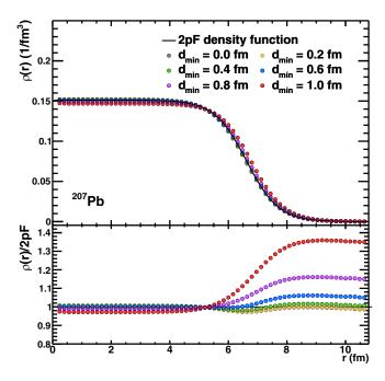
FIG. 4. Nuclear radial density distributions for various values of the internucleon distance  $d_{\min}$  using the "traditional" MCG implementation (top) and their ratio to the 2pF profile (bottom). The deviations from 1 at large *r* increase with increasing  $d_{\min}$ .
