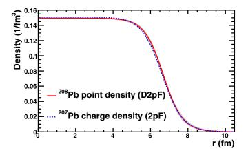
FIG. 2. Nuclear density of <sup>208</sup>Pb for the charge distribution (2pF) as well as the sum of the proton and neutron point density distributions (D2pF), corresponding to the parameters listed in Table IV. The grey band indicates the  $1\sigma$  uncertainty for the D2pF distribution.
