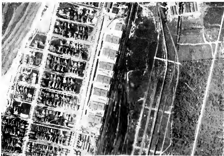
Figure 2. Same area photographed with a special American Panchromatic plate, using a red filter. (Exposure 1/30 second; altitude 10,000 feet.)
