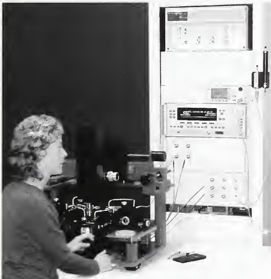
Dr. Kate Remley performs large-signal measurements of an RF power amplifier using the Nonlinear Network Measurement System.
