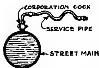
FLEXIBLE CONNECTION TO STREET MAIN.
