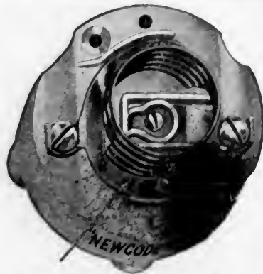
Note new way - copper shell at base turned outside, and brass yoke-pieces outside of copper shell - no close contacts to cause trouble.
