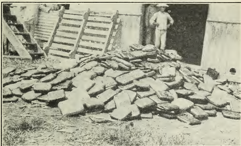
FIG. 6.—Knapsack rubber at Tres Casas, on the Madeira River. This rubber is coagulated by smoking latex over a rectangular paddle. Each knapsack represents the collection of one man for one day
