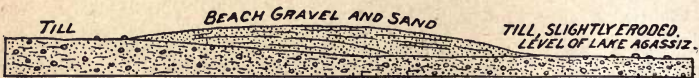
FIG. 41. Typical Section Across a Beach Ridge of Lake Agassiz. Scale, 100 feet to an inch. U. S. Geological Survey.
