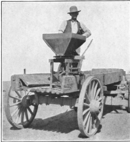
FIG. 1.—BROADCAST GRAIN SEEDER ATTACHED TO WAGON USED IN SOWING POISONED BRAN BAIT.
