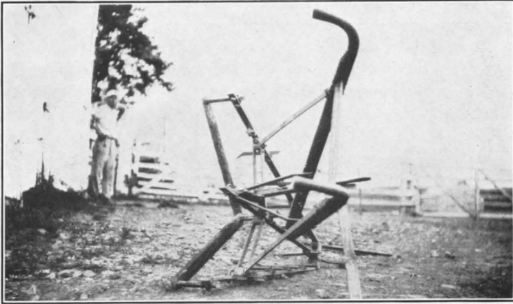
FIG. 1.—ATTACHMENT FOR ORCHARD HARROW INVENTED BY COUNTY AGENT. Over 1,000 of these are in use in Christian County, Ky. Note the weed-cutting bar attached to back cultivator teeth.
