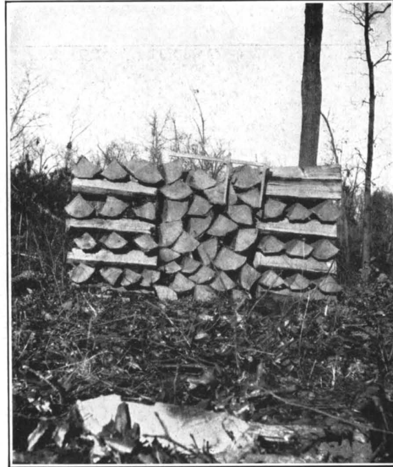
FIG. 2.—WHITE OAK STAVE BOLTS FOR TIGHT COOPERAGE PILED TO ALLOW FREE CIRCULATION OF AIR.
