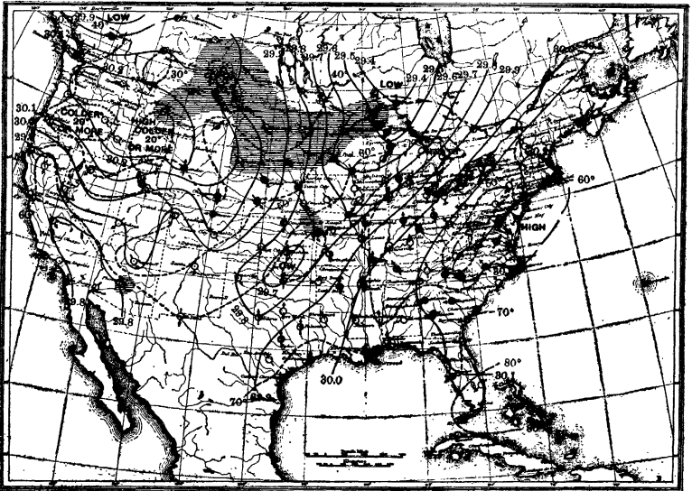
FIG. 11.—Weather map, September 26, 1903, the first of a series of three, showing progress of weather changes across the country. The solid lines run through points of equal atmospheric pressure; the broken lines run through points of equal temperature; the circles show state of weather, white for clear, black for cloudy; arrows point in direction wind is blowing; shaded areas show regions of precipitation last 24 hours.
