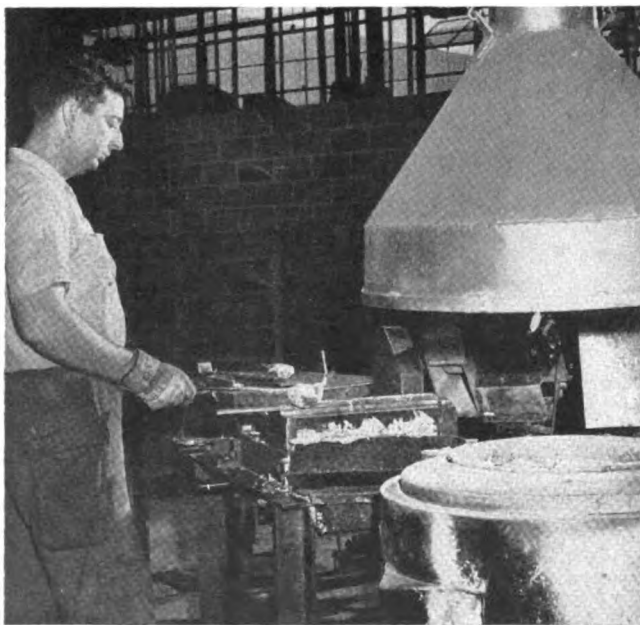
1. The operation of terminal and strap molding in the photograph is well-ventilated. Note the section in the duct which the worker can lower about 15 inches when necessary. The shield at the back serves to decrease cross drafts.
