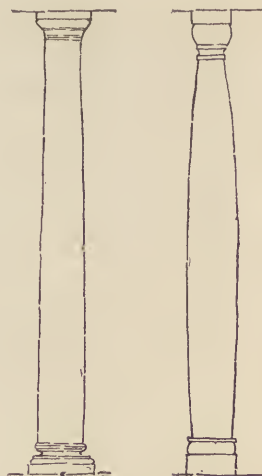
Architect's turned post.
