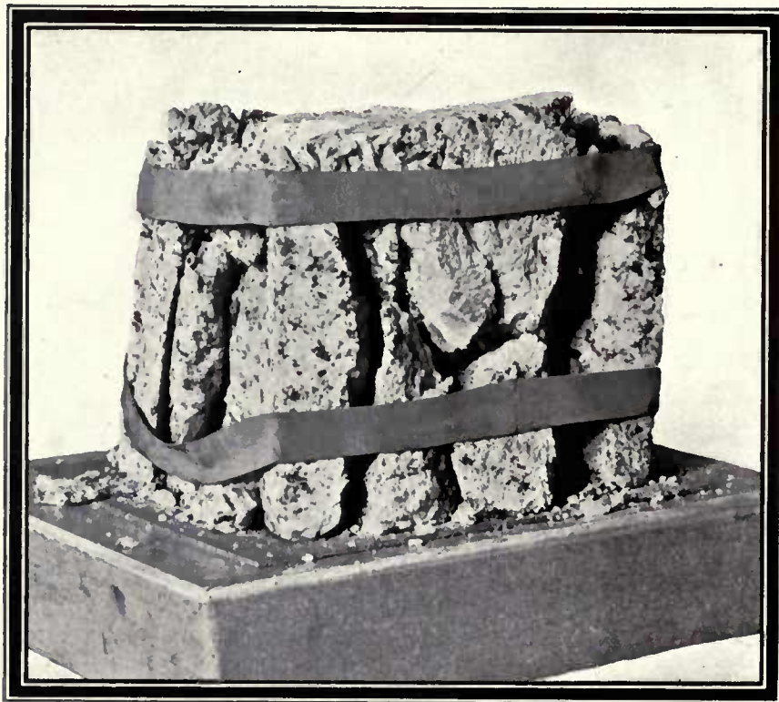
TENTERFIELD GRANITE, N.S.W. 3 IN. CUBE CRUSHED AT 54.18 TONS (J. NANGLE)
