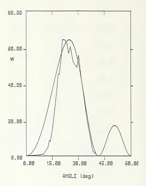
Figure 36 Cerenkov Radiation Data From Figure 24 Compared with Theoretical Curves where L=14.0 cm and the Angular Shift is +7.0 Degrees
