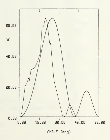
Figure 30 Cerenkov Radiation Data From Figure 26 Compared with Theoretical Curves where L=14.0 cm and the Angular Shift is 0.0 Degrees
