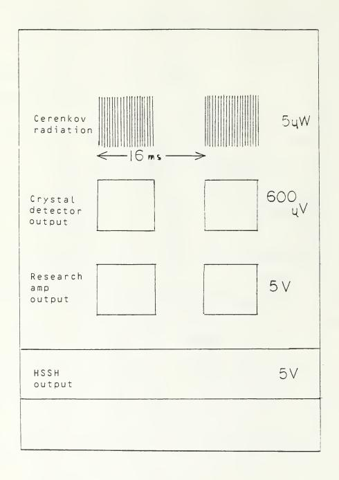
Figure 18 Signal Morphology from Beam to X/Y Recorder
