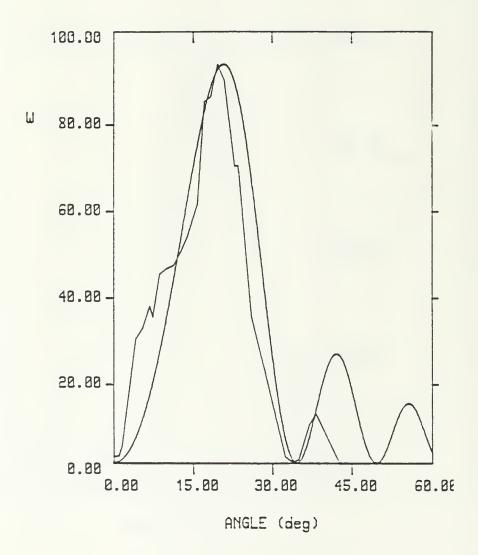
Figure 34 Cerenkov Radiation Data From Figure 26 Compared with Theoretical Curves where L=20.0 cm and the Angular Shift is 0.0 segrees
