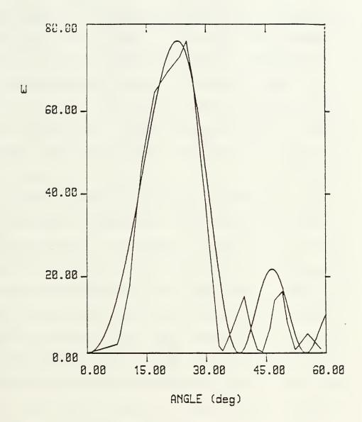
Figure 39 Cerenkov Radiation Data From Figure 27 Compared with Theoretical Curves where L=16.5 cm and the Angular Shift is +7.5 Degrees
