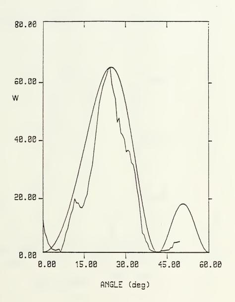
Figure 37 Cerenkov Radiation Data From Figure 25 Compared with Theoretical Curves where L=14.0 cm and the Angular Shift is +5.4 Degrees
