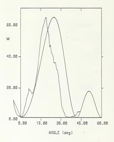
Figure 29 Cerenkov Radiation Data From Figure 25 Compared with Theoretical Curves where L=14.0 cm and the Angular Shift is 0.0 Degrees
