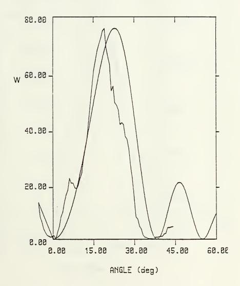
Figure 33 Cerenkov Radiation Data From Figure 25 Compared with Theoretical Curves where L=16.5 cm and the Angular Shift is 0.0 Degrees
