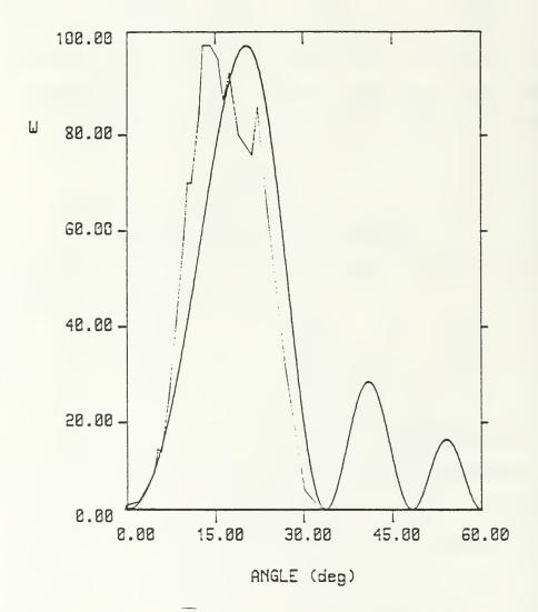
Figure 32 Cerenkov Radiation Data From Figure 24 Compared with Theoretical Curves where L=21.0 cm and the Angular Shift is 0.0 Degrees
