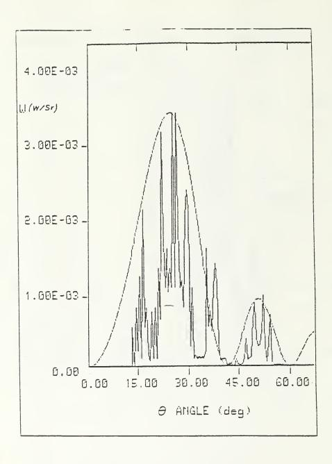
Figure 10 Vujaklija's Data using the Mirror for the Third Harmonic with an angular shift of 13 degrees
