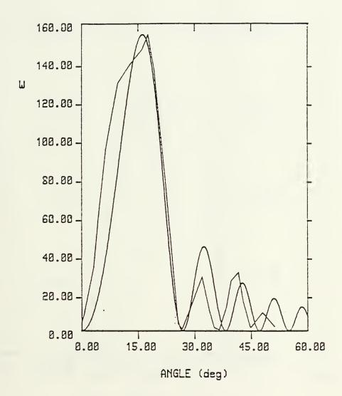
Figure 35 Cerenkov Radiation Data From Figure 27 Compared with Theoretical Curves where L=33.0 cm and the Angular Shift is 0.0 Degrees
