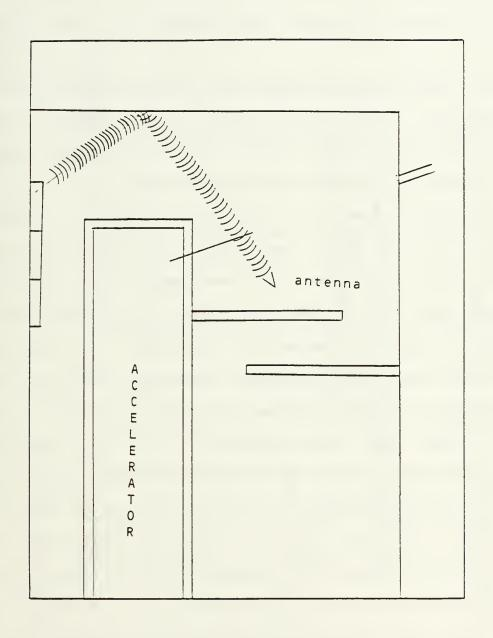
Figure 21 Antenna Position for Measuring Klystron Noise
