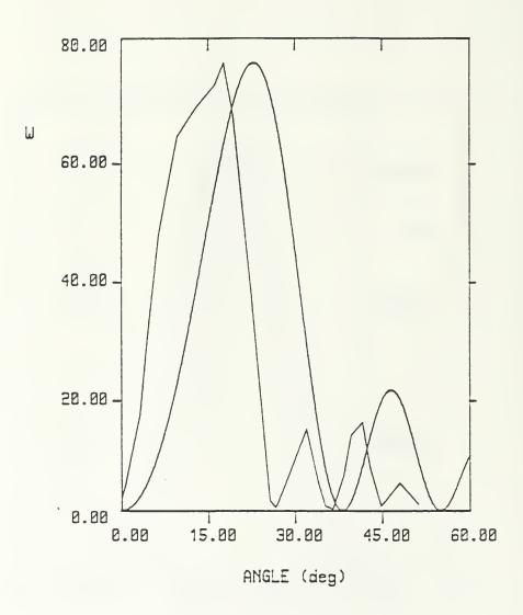
Figure 31 Cerenkov Radiation Data From Figure 27 Compared with Theoretical Curves where L=16.5 cm and the Angular Shift is O.O Degrees
