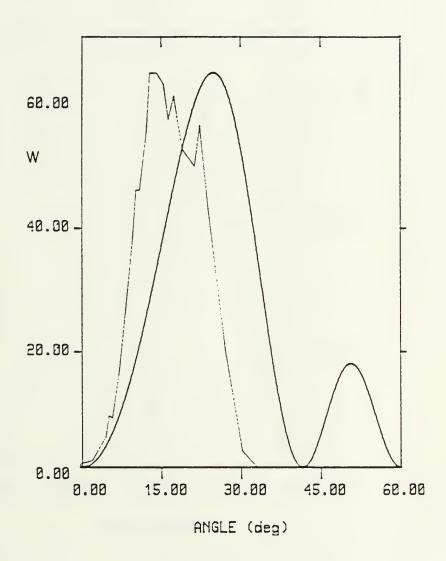
Figure 28 Cerenkov Radiation Data From Figure 24 Compared with Theoretical Curves where L=14.0 cm and the Angular Shift is 0.0 Degrees
