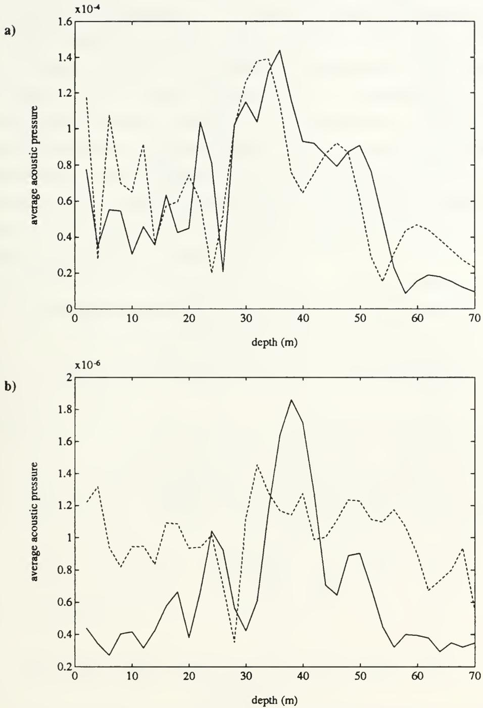
**Fig 12. Depth dependence of average acoustic pressure for a 5 kHz source at range a) 20 km and b) 100 km. The source is at 35 m depth in the surface duct. Solid lines show average acoustic pressure in a temperature invariant OML. Dashed lines show average acoustic pressure in a temperature varying OML.**
