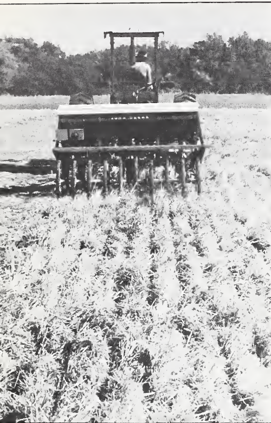
Lo-Till, an educational/research program, has become synonymous with minimum tillage in Oklahoma. Here, a wheat drill works its way through last season's stubble.
