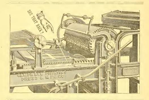
Showing the new Register Rack, FULL LENGTH OF THE IMPRESSION SURFACE.
