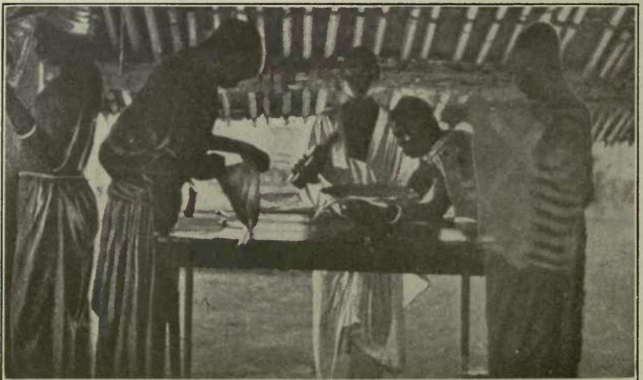
FIG. 11—COAGULATION OF LATEX AND PREPARING SHEETS
