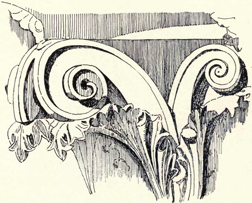
FIG. 34. DETAILS OF VOLUTES FROM CAPITAL, TEMPLE OF VESTA, ROME, AFTER D'ESPOUY
