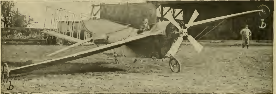
3. THREE-QUARTERS VIEW OF THE ESNAULT-PELTERIE MONOPLANE. The wing wheels b b and the twisting rudder h are features of this machine.
