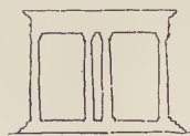
240. The same, with intermediate columns moved toward the centre, leaving double openings.
