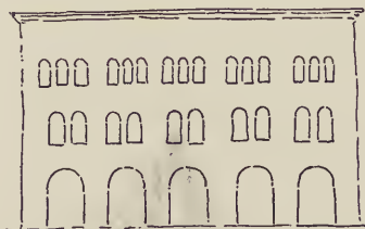
152. Variation of openings in spite of the continuity of the piers.
