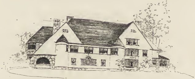
255. Double unsymmetrical group of gables, with an additional double symmetrical group of turrets.
