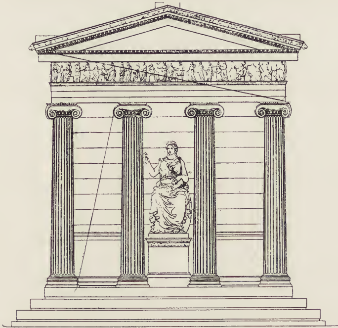
189. Temple of Nike Apteros. Diagonals show relation of intercolumniation to entablature.
