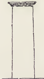
181. Bad effect of cornice of heavy projection on a tall and narrow front.
