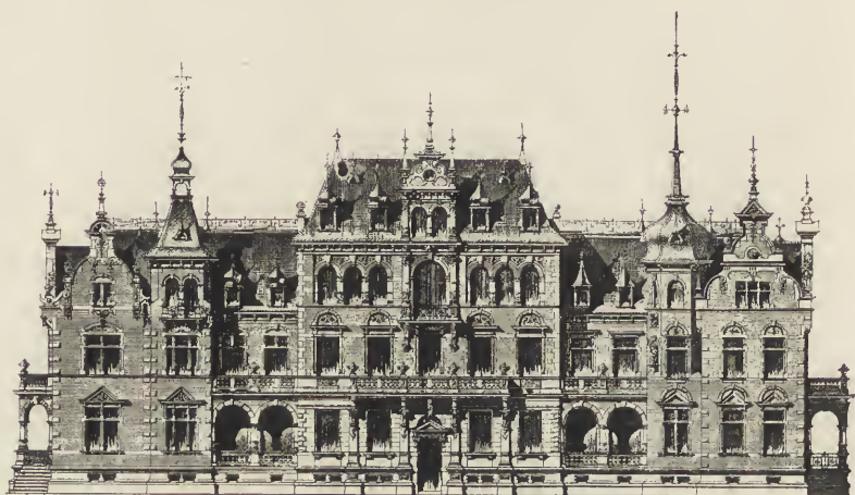
246. A Double Private House in Heidelberg. The entire lack of symmetry in the lateral members does not in the least detract from the sense of triplicity in the group.
