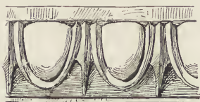
Fig. 20. Carved egg-and-dart moulding, from Erechtheum, 5th century B. C.
